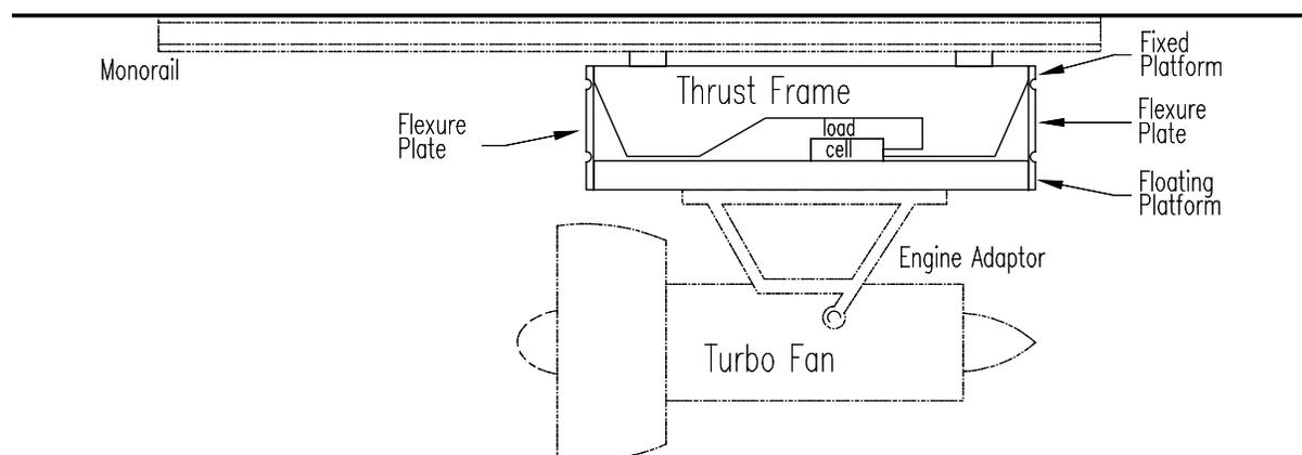
**FIGURE 2-4. TYPICAL THRUST MOUNT DESIGN**
