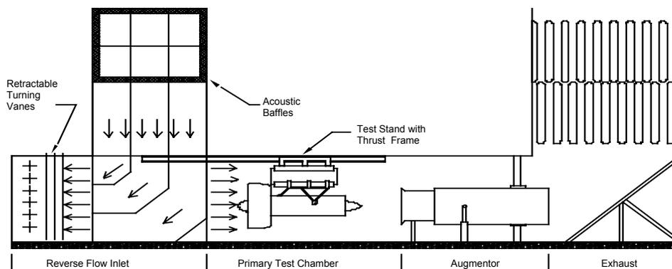
**FIGURE 2-3. TEST CELL CONFIGURATION: FOLDED INLET TYPE**
