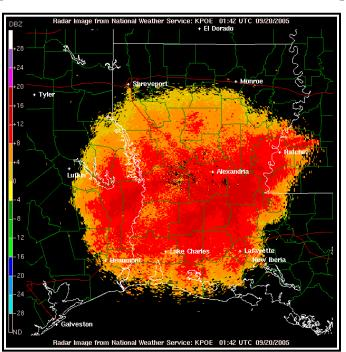
Figure 3-23. WSR-88D Weather Radar Ghost Example
