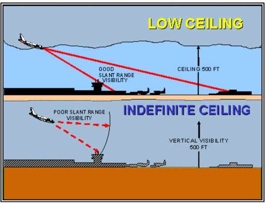
Figure 3-3. Obscuration Effects on Slant Range Visibility
