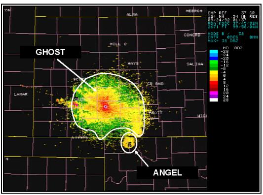
Figure 3-24. WSR-88D Weather Radar Angel Example
