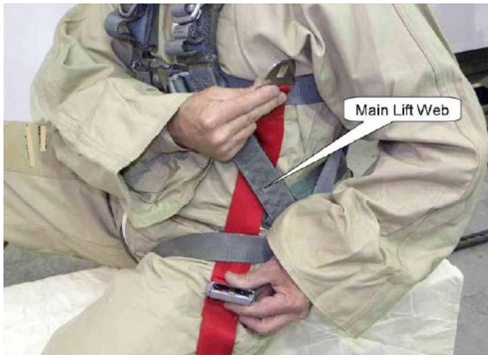
FIGURE 5. PASS TETHER LOOP UNDER MAIN LIFT WEB
