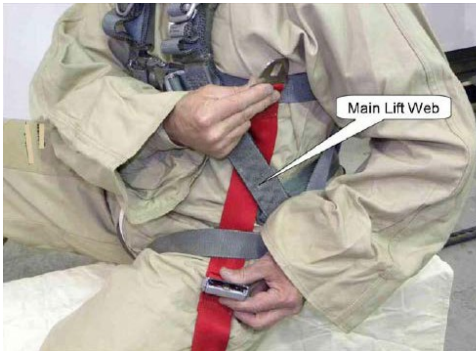
FIGURE 5. PASS TETHER LOOP UNDER MAIN LIFT WEB
