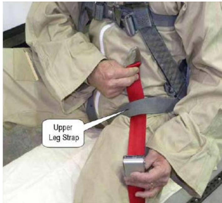
FIGURE 5. PASS TETHER LOOP UNDER MAIN LIFT WEB
