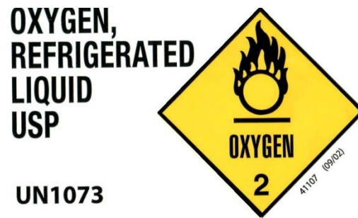
Figure 1. Example of Hazmat Labeling
