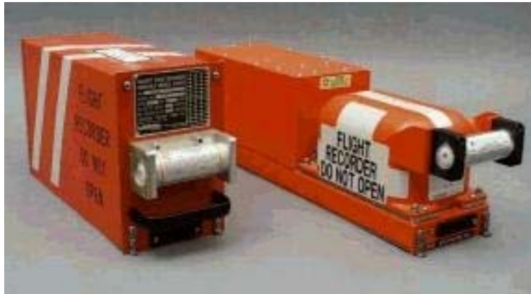
Figure 1. Representative Flight Data Recorders
