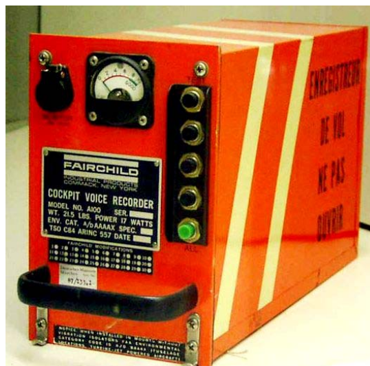
Figure 2. Representative Cockpit Voice Recorder
