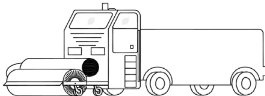
Pushed type sweeper special purpose or truck type vehicle two engine/front blower heavy duty/large swath
