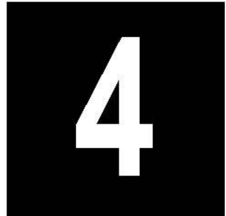
Figure 3. Runway Distance Remaining Sign (RDR). An RDR is Type L-858B, with a white legend on a black background and conforming to AC 150/5345-44, Size 4, Style 2 or 3.
