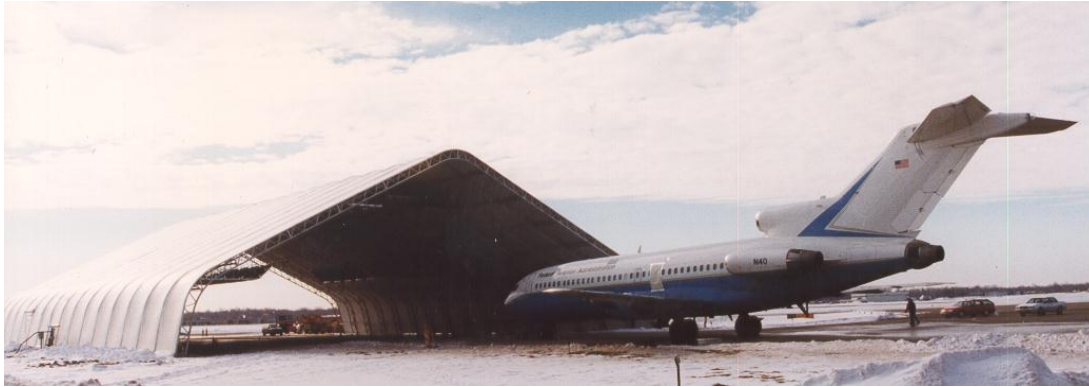
Figure 5-2. FAA Boeing 727-100 taxiing into an infra-red deicing structure test site
