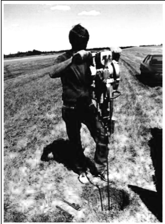
Figure 8.20. Driving the stainless steel rod to refusal.
