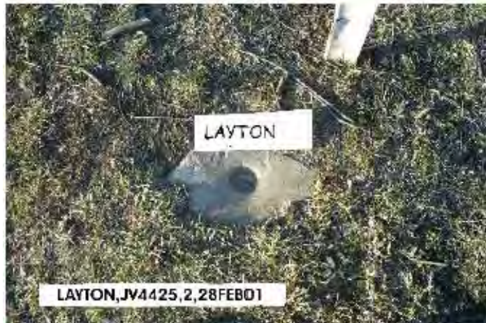
Figure 8.5. Example of the NGS suggested Type 2 digital photograph.
