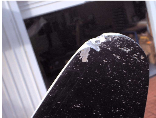
FIGURE 1-13. Propeller Blade Struck by a Foreign Object
