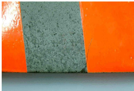
FIGURE 1-9. Blade Crack From a Nick
