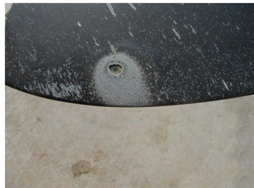
FIGURE 1-12. Lightning Strike on a Composite Surface
