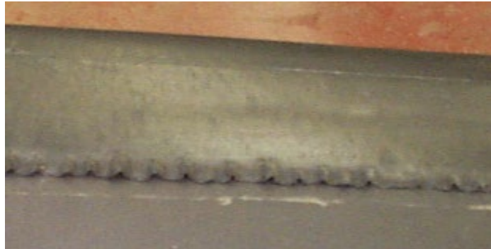
FIGURE 2-3. Heater Edge Debond
