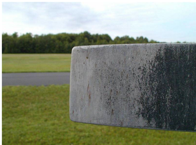
FIGURE 1-7. Erosion on a Metal Blade
