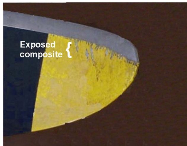
FIGURE 2-6. Composite Blade Erosion
