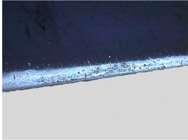
FIGURE 1-5. Exfoliation on the Blade Leading Edge
