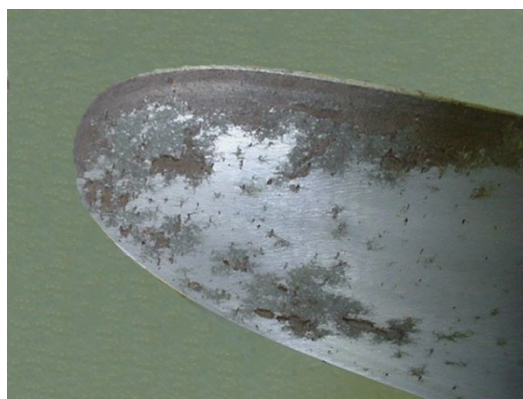
FIGURE 1-2. Polished Blade Surface Corrosion
