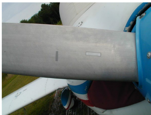
FIGURE 3-1. Balance Tape That Was Not Removed
