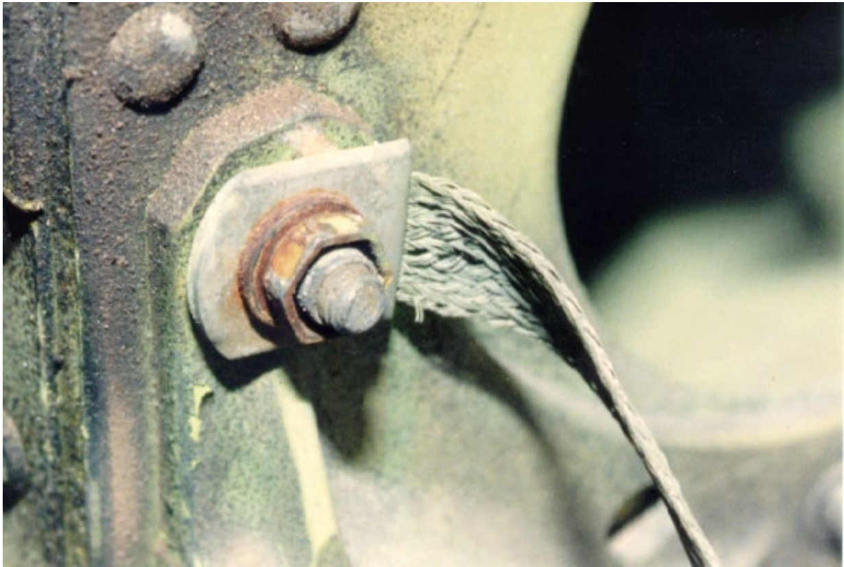
FIGURE 6-7. CORRODED BONDING STRAP AND ATTACH HARDWARE
