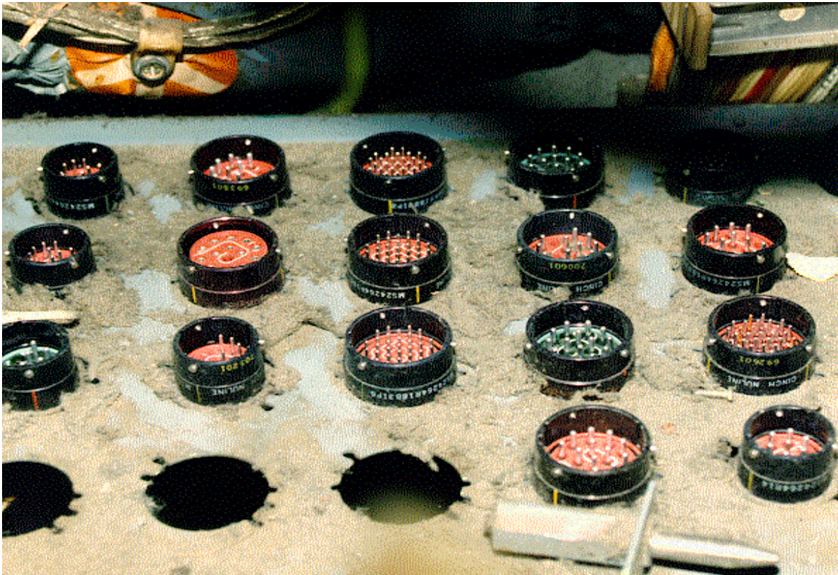
FIGURE 6-6. LINT AND DEBRIS ACCUMULATION ON A SHELF
