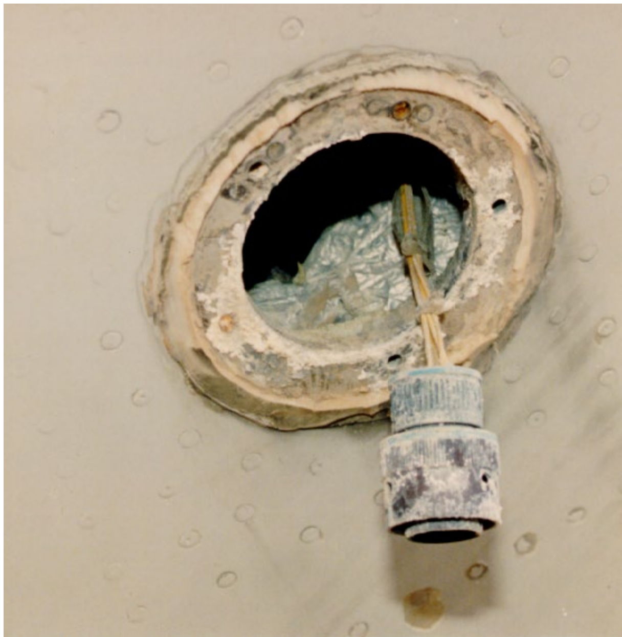
FIGURE 6-8. CORRODED ANTENNA MOUNTING AREA AND ELECTRICAL PLUG
