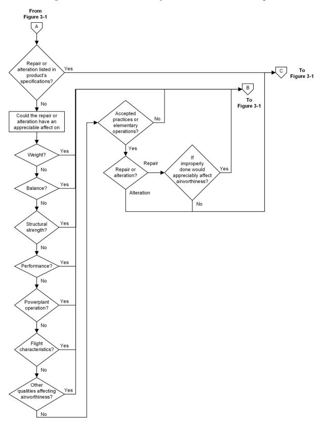
Figure 3-2. Determination of Major or Minor Alteration or Repair
