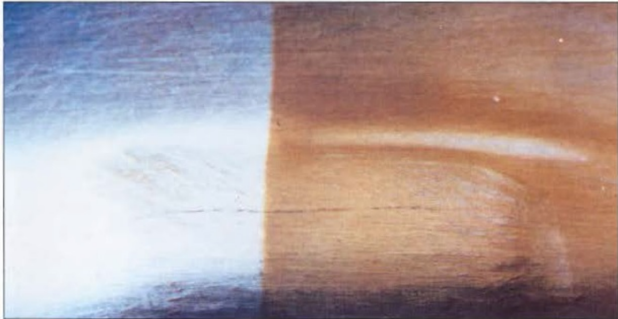
Figure 5-18. Alodine 1200 Treatment Prior to Painting May Highlight Presence of Remaining Corrosion or Cracks
