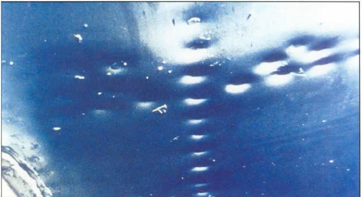
Figure 5-5. Skin Bulging Around Fasteners Caused by Pressure from Corrosion Products
