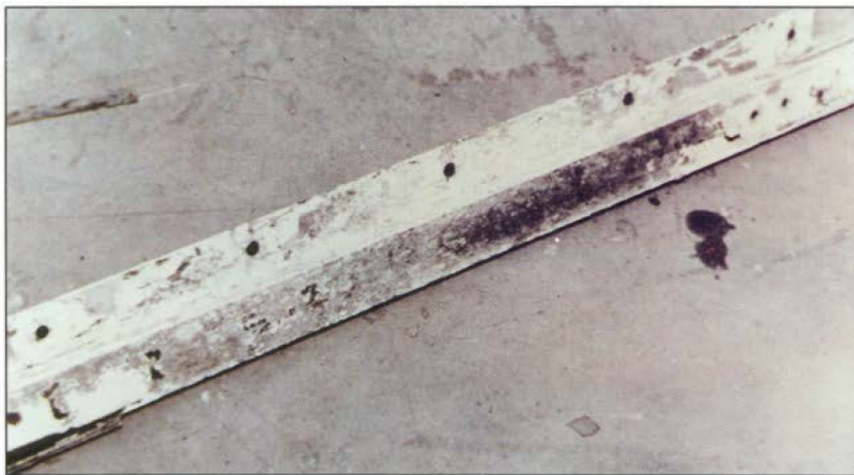
Figure 2-3. Uniform Etch Corrosion
