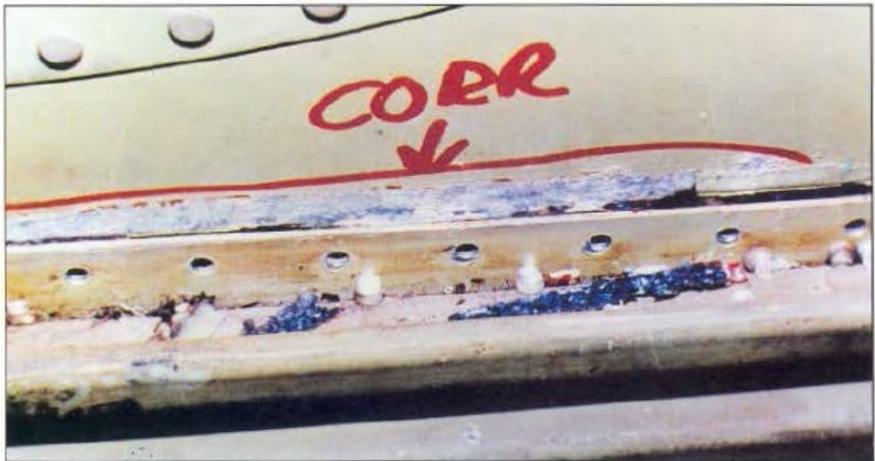
Figure 5-11. Removal of Insulation Blankets Exposed Corrosion
