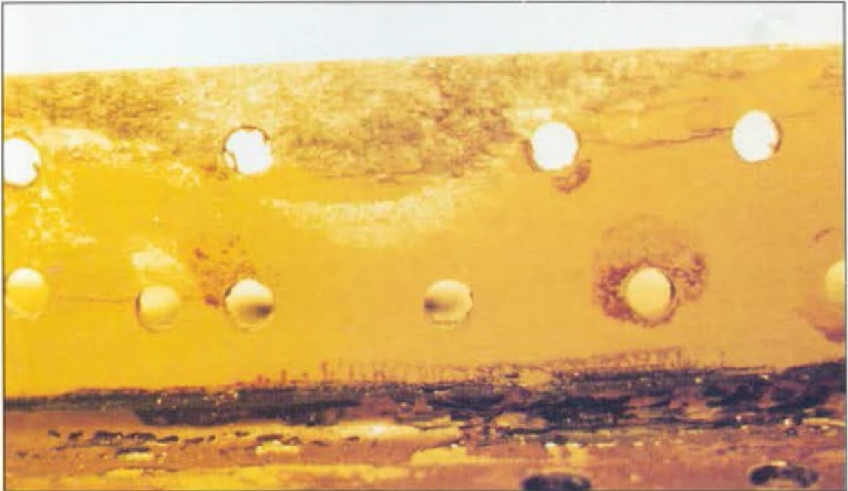
Figure 5-7. Faying Surface Corrosion on Wing Spar Chord with Corrosion Cracking Also Visible
