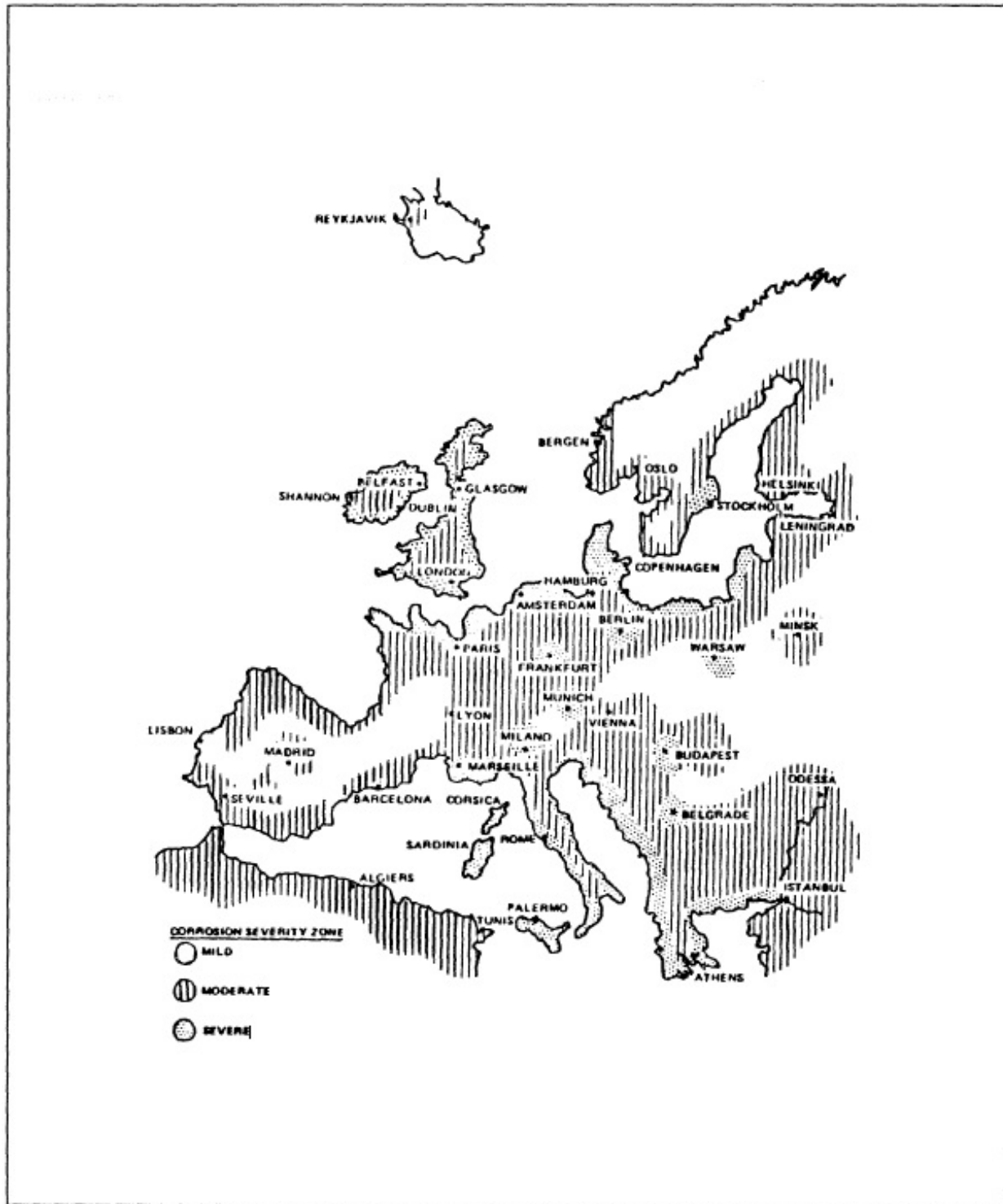
Figure 4-20. Europe and Asia Minor Corrosion Severity Map
