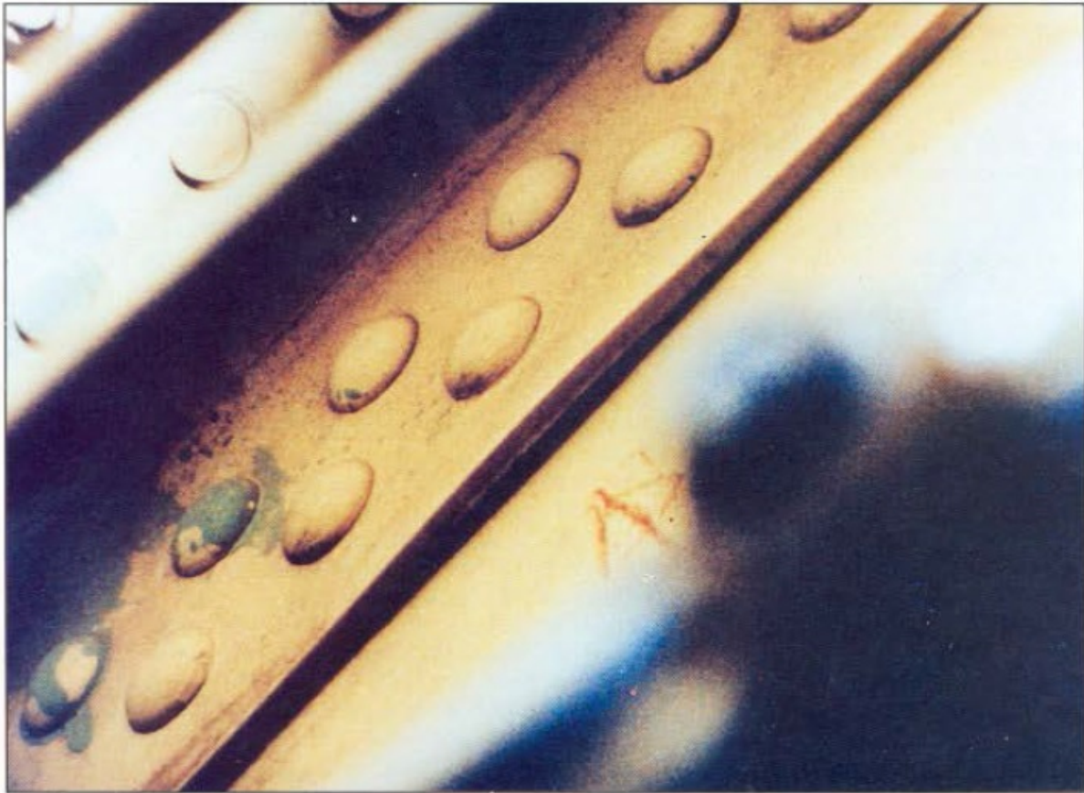
Figure 4-12. Skin Bulging Around Fasteners
