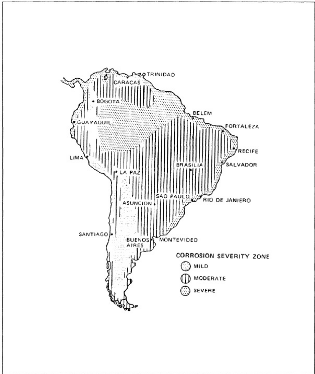
Figure 4-16. South America Corrosion Severity Map
