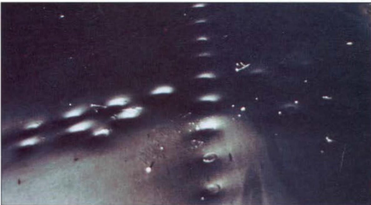
Figure 4-12. Skin Bulging Around Fasteners
