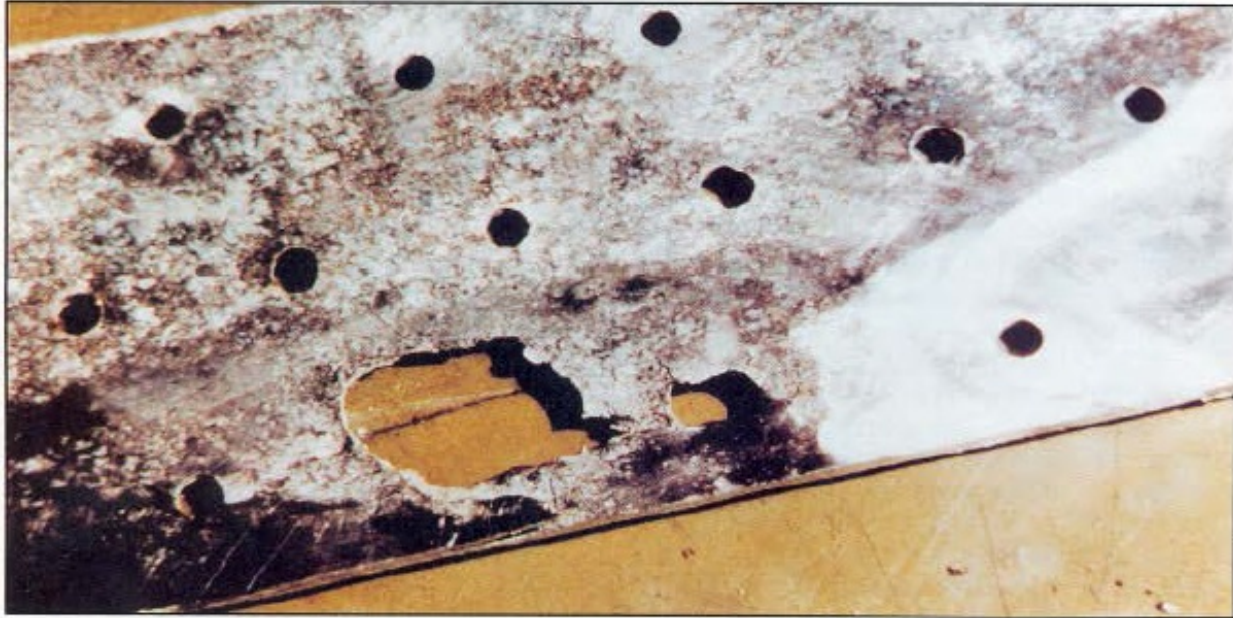
Figure 6-9. Corrosion at Fastener Holes Removed by Spot Facing
