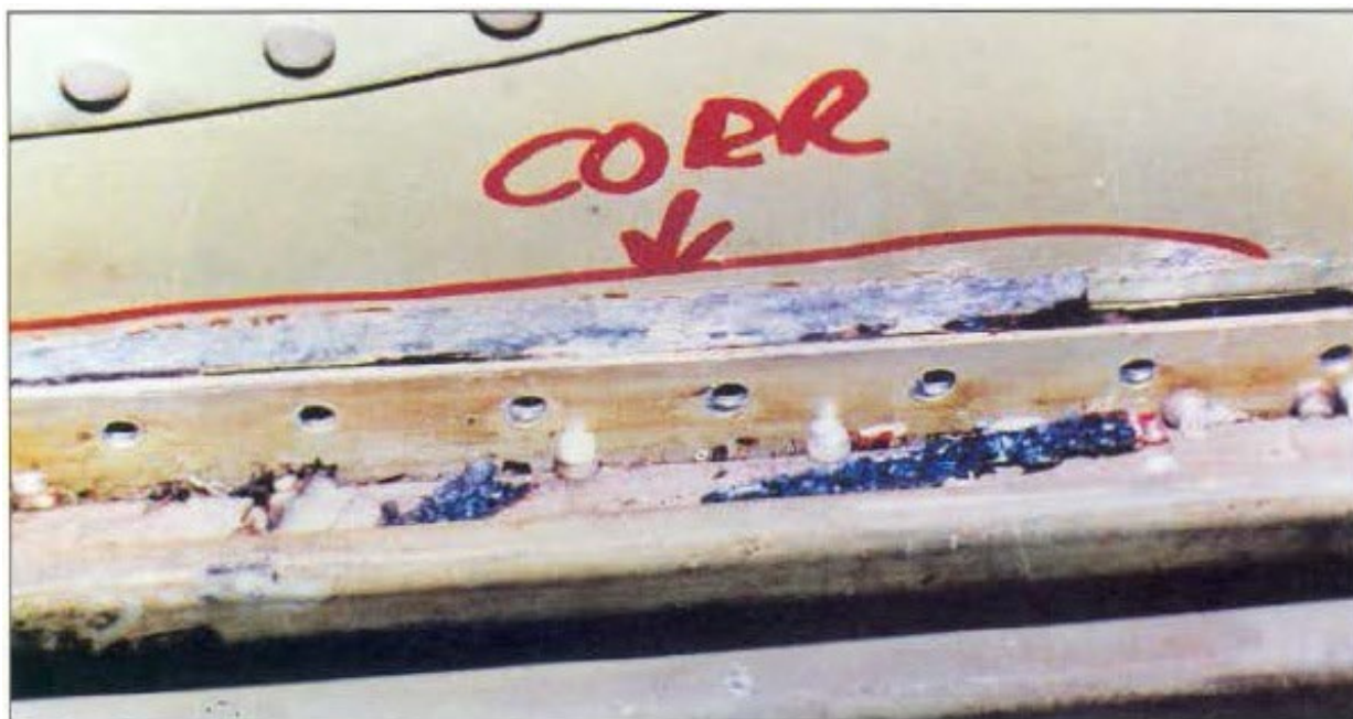
Figure 5-11. Removal of Insulation Blankets Exposed Corrosion
