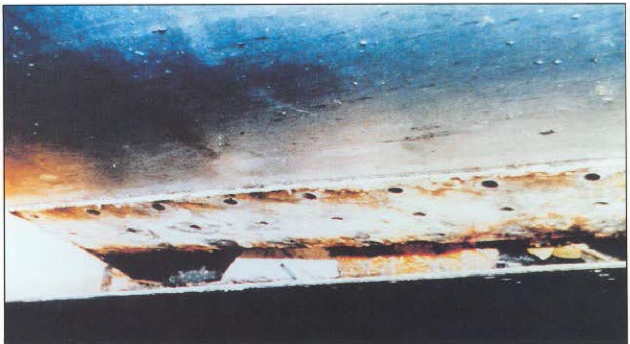
Figure 5-15. Severely Corroded Lap Joint
