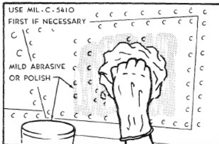
Figure 6-12. Polishing and Brightening Alclad Surfaces
