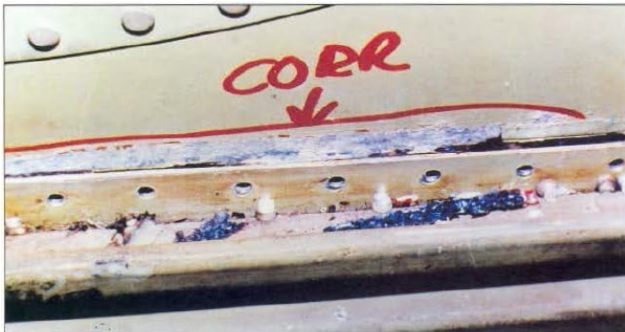
Figure 5-11. Removal of Insulation Blankets Exposed Corrosion
