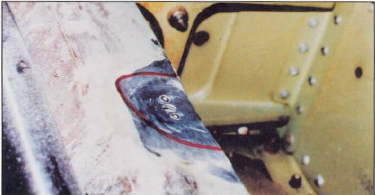
Figure 6-5. Steel Particles from Fasteners or Nutplates May Cause Future Corrosion Problems in Aluminum Structure
