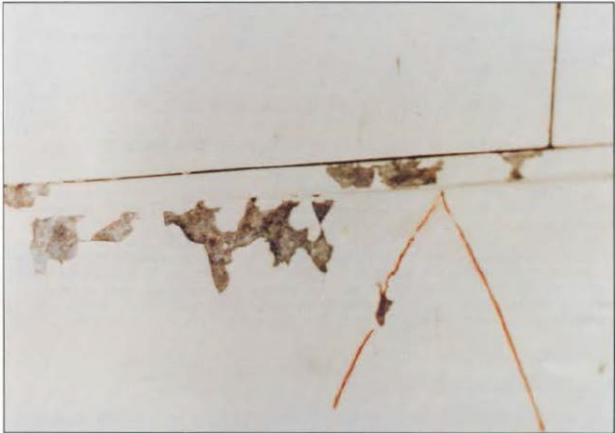
Figure 5-3. Corrosion Indicated by Blistering of Paint in Fuel Cell
