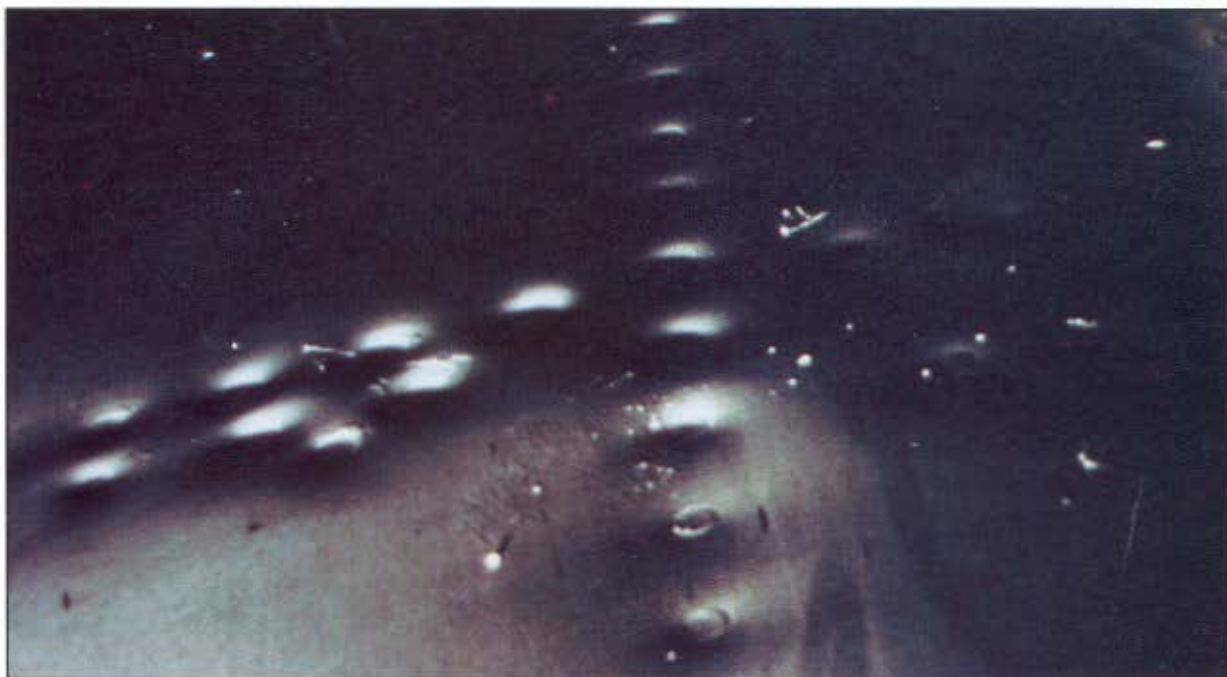
FIGURE 4-12. SKIN BULGING AROUND FASTENERS
