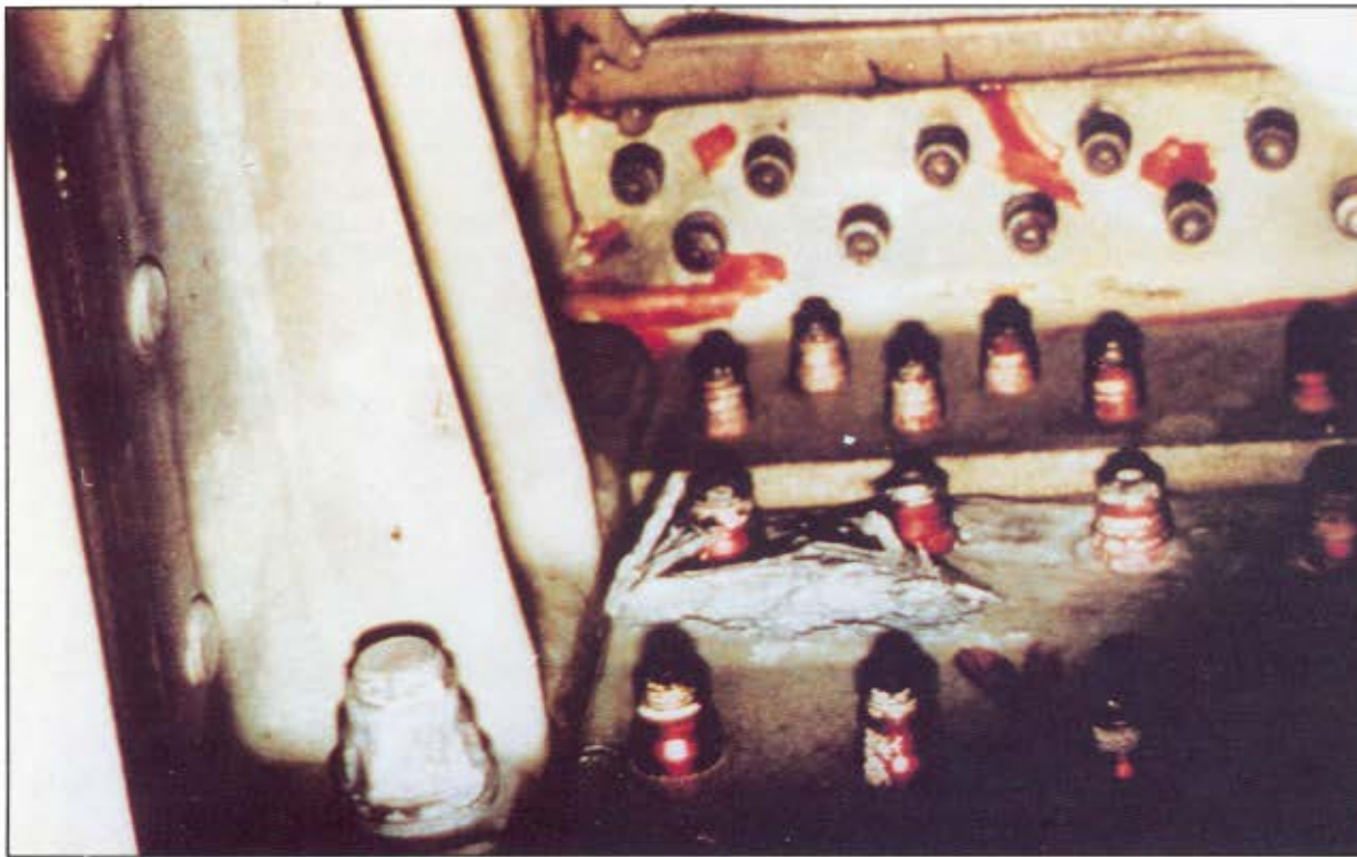
FIGURE 2-9. SEVERE EXFOLIATION CORROSION
