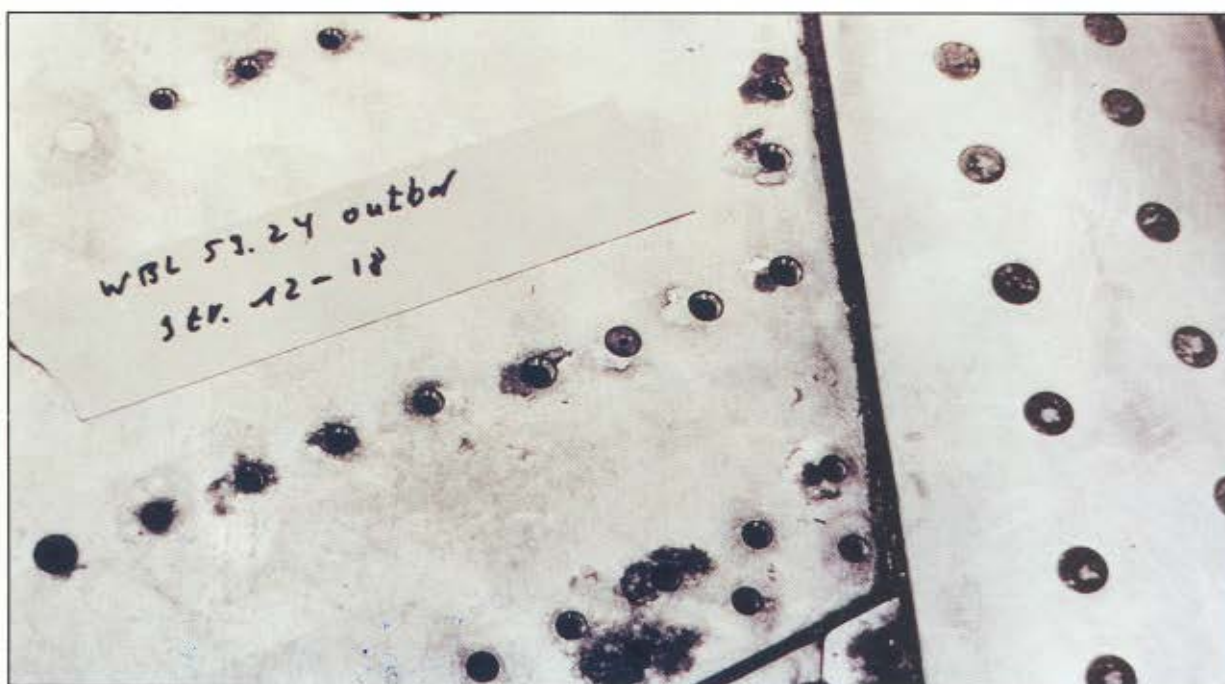
FIGURE 5-14. CORROSION DAMAGE AROUND FASTENER HOLES AND IN FASTENER HOLES
