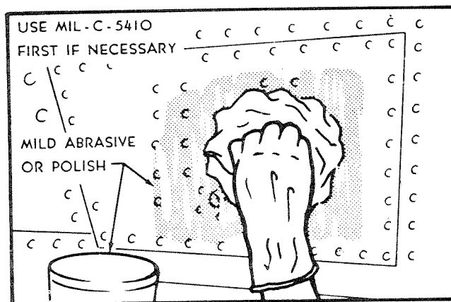
FIGURE 6-12. POLISHING AND BRIGHTENING ALCAD SURFACES
