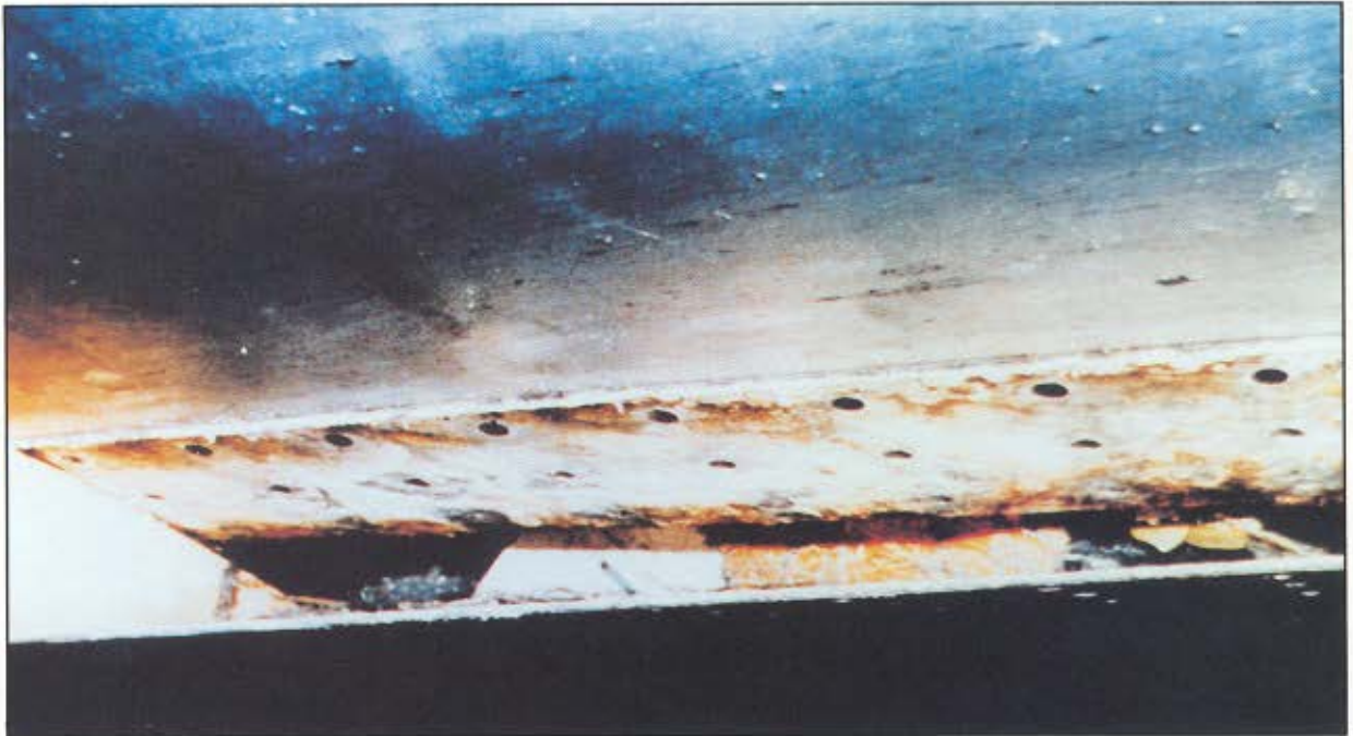
FIGURE 5-15. SEVERELY CORRODED LAP JOINT
