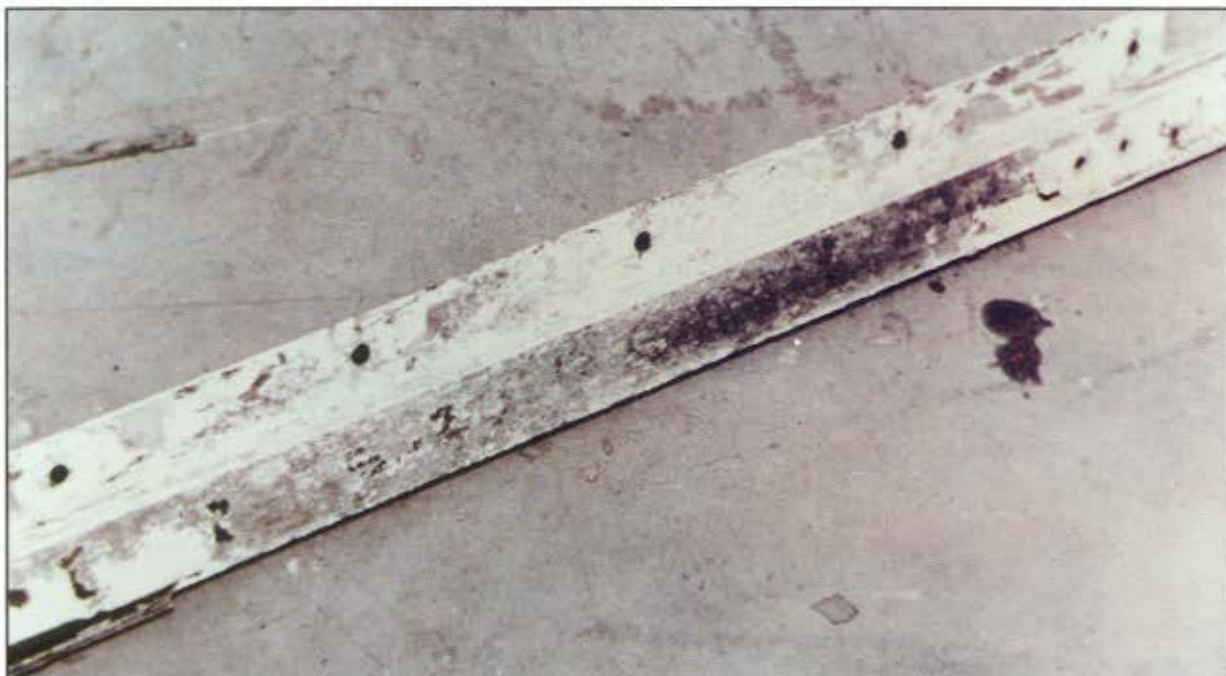
FIGURE 2-3. UNIFORM ETCH CORROSION
