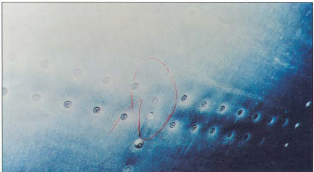
FIGURE 5-4. POPPED RIVET HEADS RESULTING FROM CORROSION PRODUCTS
