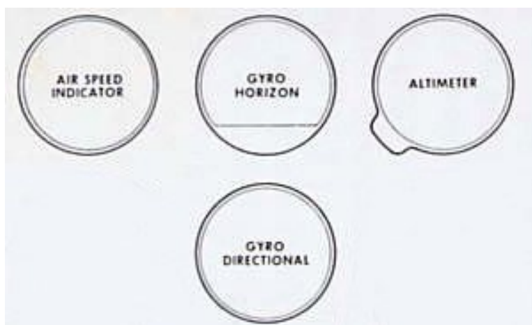
Figure 12-1. The Basic “T” Visual Meteorological Conditions (VMC) Instrument Configuration
