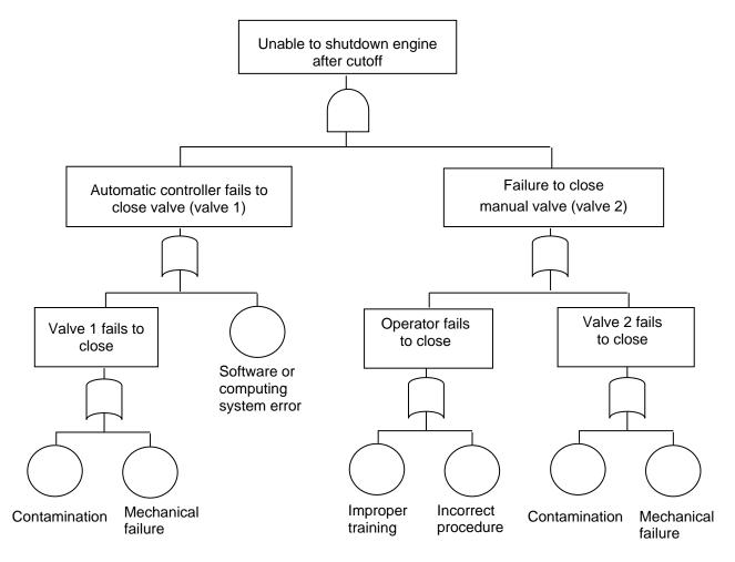
**Figure B-1 Fault Tree for Engine Shutdown Failure.**
