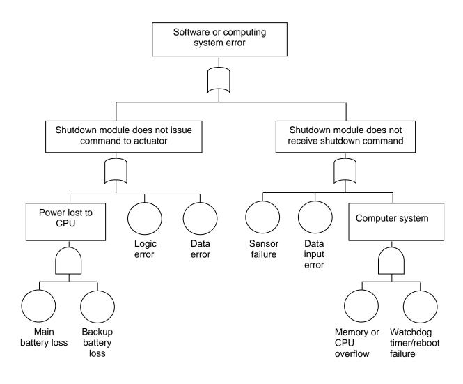
Figure B-2 Fault Tree for Software or Computing System Errors
