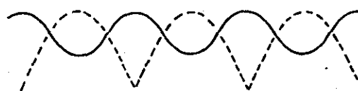
FIGURE 8-248. Output of an inductor filter rectifier.
