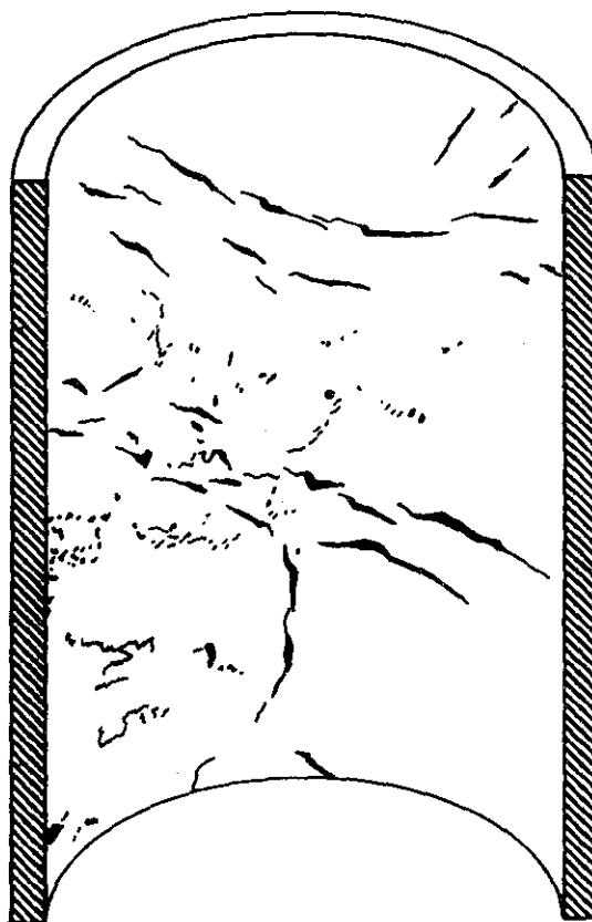
FIGURE 10-9. Heat-treat cracks on cylinder barrel wall.
