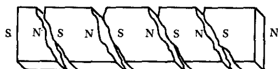
FIGURE 8-89. Magnetic poles in a broken magnet.
