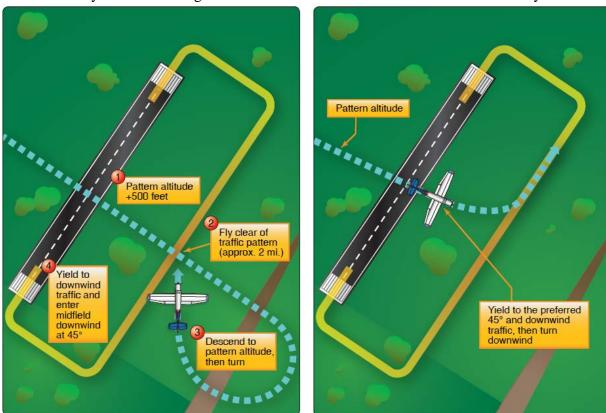
11.4 Traffic Pattern Altitudes. It is recommended that airplanes observe a 1,000 foot above ground level (AGL) traffic pattern altitude. Large and turbine-powered airplanes should enter the traffic pattern at an altitude of 1,500 feet AGL or 500 feet above the established pattern altitude. Ultralight aircraft should operate no higher than 500 feet below the powered aircraft pattern altitude. A pilot may vary the size of the traffic pattern depending on the aircraft's performance characteristics.
