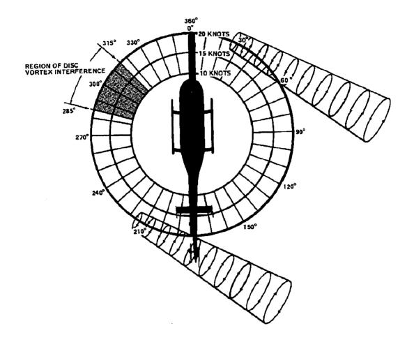
FIGURE 1. MAIN ROTOR DISC VORTEX INTERFERENCE
