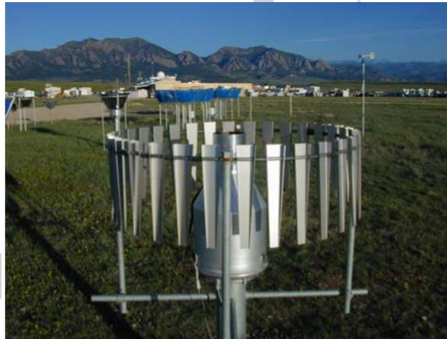
Figure 3-1. ETI Precipitation Gauge in a Single Alter Wind Shield 2 Type
