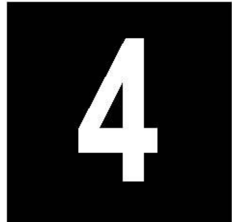
Figure 3. Runway Distance Remaining Sign (DRS). A DRS is Type L-858B, with a white legend on a black background and conforming to AC 150/5345-44, Size 4, Style 2 or 3.
