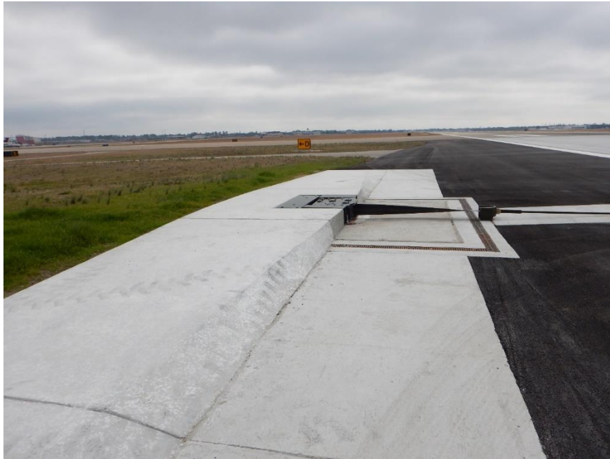
Figure A-13. Figure A2-5. Edge Sheave and Ramp (Side View)
