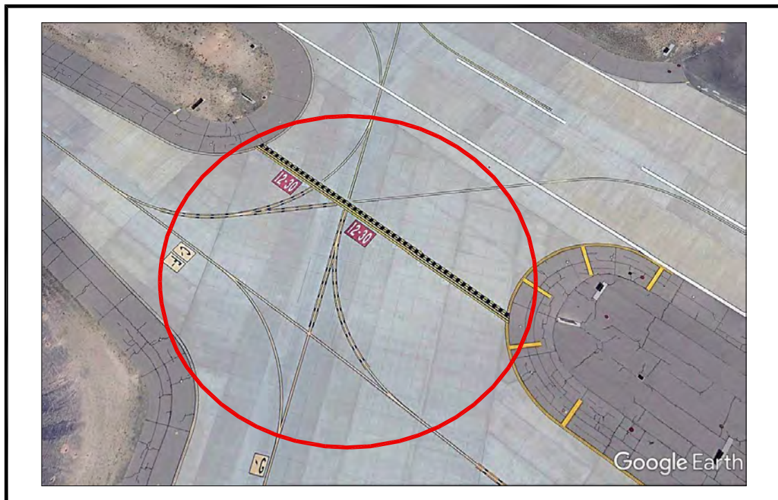
Figure J-17. Aerial Image of Complex Taxiway Intersection Exceeding the “Three-Path” Concept
