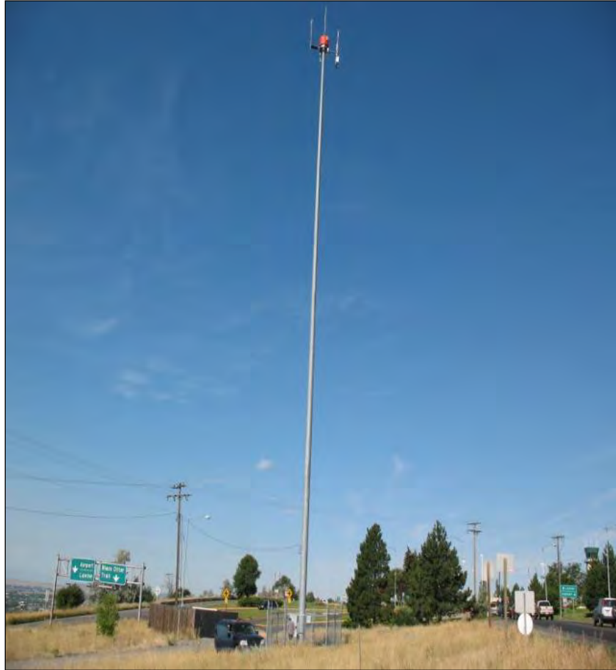
Figure 6-28. Low Level Windshear Alert System (LLWAS) Sensor Pole
