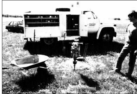
Figure 7-9. Shows the NGS Mark Setting Truck and associated equipment.
