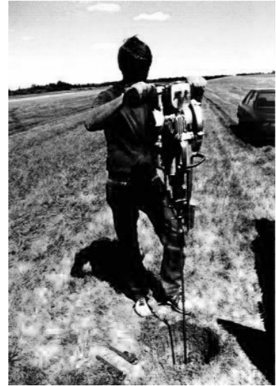
Figure 7-14. Driving the stainless steel rod to refusal.
