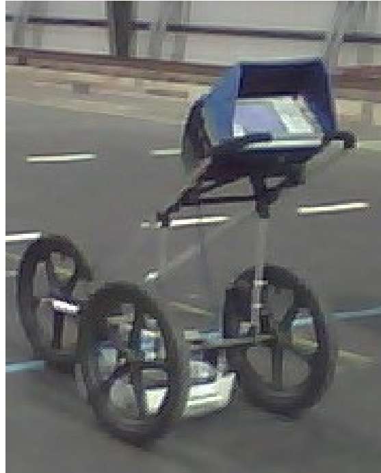
Figure E-2. Cart based GPR (NAPTF)
