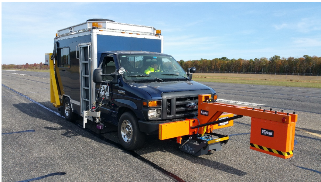
Figure E-1. Vehicle based Air-Coupled GPR (NAPTF)
