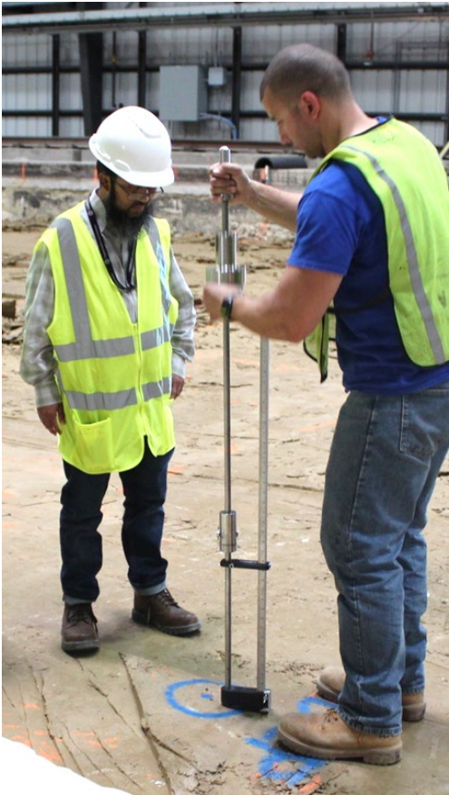
Figure D-2. DCP in Use (NAPTF)
