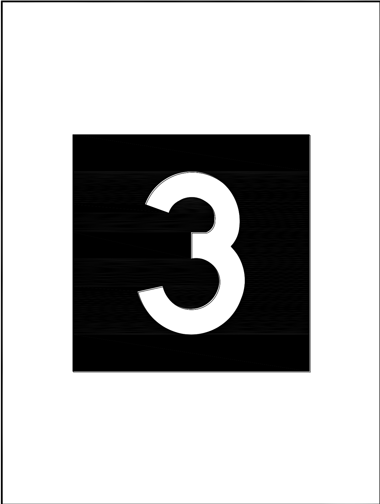
Figure 2-20. Runway Distance Remaining Sign.
