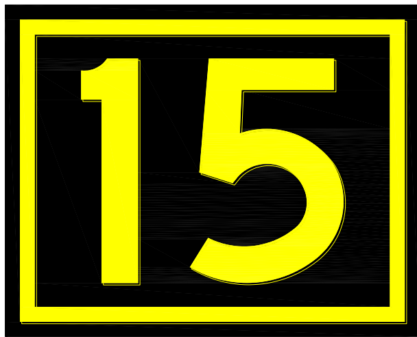
(b) Runway Location Sign
