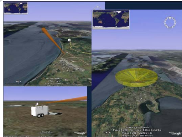
(b) Representations of Dish Antenna Coverage as a Single Cone (Left) and the Full Volume Covered as the Dish Rotates (Right)
