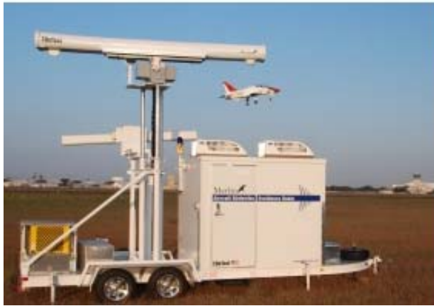
(a) A slotted array antenna
