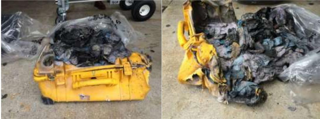
This item had undeclared lithium batteries installed as a power source in equipment. This is an example of a thermal runaway of lithium batteries.
