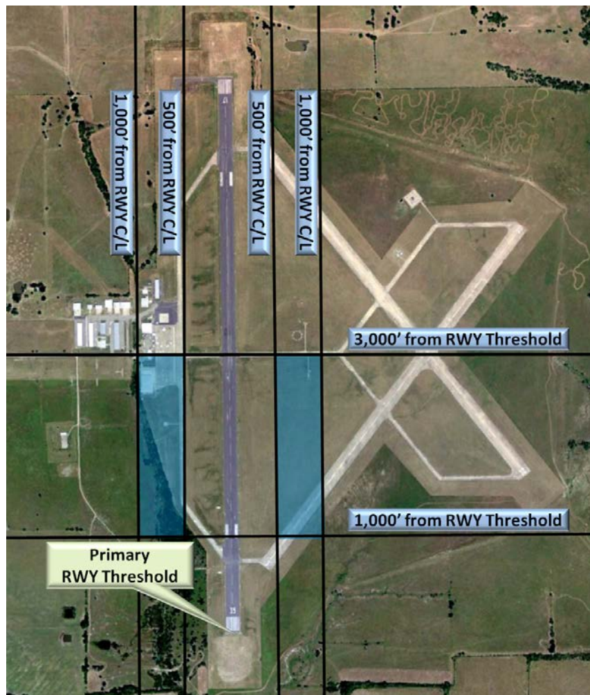
Figure 3-1. Siting Criteria for Airports with Only Visual and/or Non-Precision Runways
