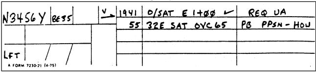
FIG 4-2-5 Flight Progress Strip
