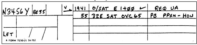
FIG 4-2-5 Flight Progress Strip
