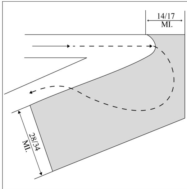
d. After the course changes specified in subparagraphs b or c have been completed and the aircraft is back on course, the appropriate minima in subparagraph a may be used.
