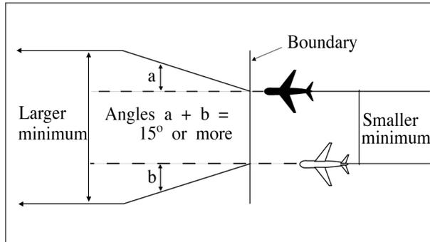
b. Intersecting flight paths with constant and same width protected airspace when either aircraft is at or beyond a distance equal to the applicable lateral separation minimum measured perpendicular to the flight path of the other aircraft. (See FIG 8-4-4.)
