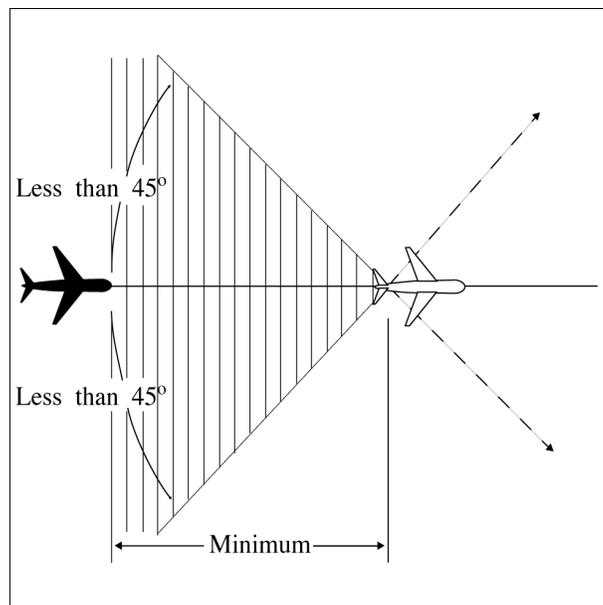
2. **Crossing tracks.** Ensure that the estimated spacing at the point of intersection is not less than the applicable minimum required. (See FIG 8-3-2.)
