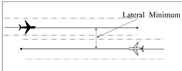
2. When reduced route protected airspace is applicable, and the protected airspace of the flight paths do not overlap; or (See FIG 8-4-2.)
