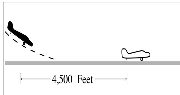
2. The other aircraft has departed and crossed the runway end. (See FIG 3–10–4). If you can determine distances by reference to suitable landmarks and the other aircraft is airborne, it need not have crossed the runway end if the following minimum distance from the landing threshold exists:
