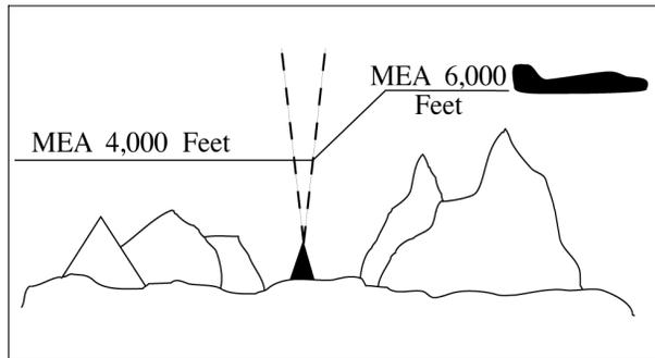
2. If a MCA is specified, prior to the fix so as to cross the fix at or above the MCA. (See FIG 4-5-2)
