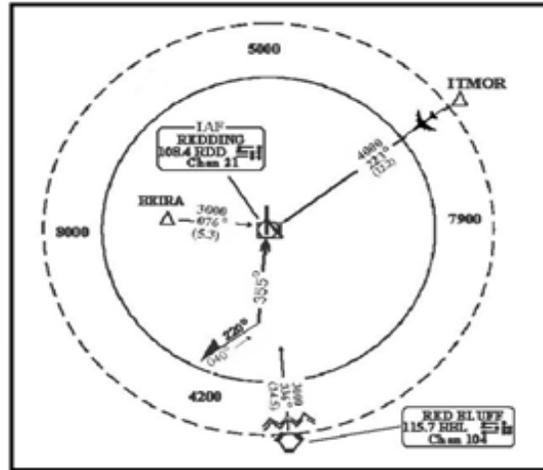
2. Assigned an altitude to maintain until the aircraft is established on a segment of a published route or instrument approach procedure. (See FIG 4-8-2.)
