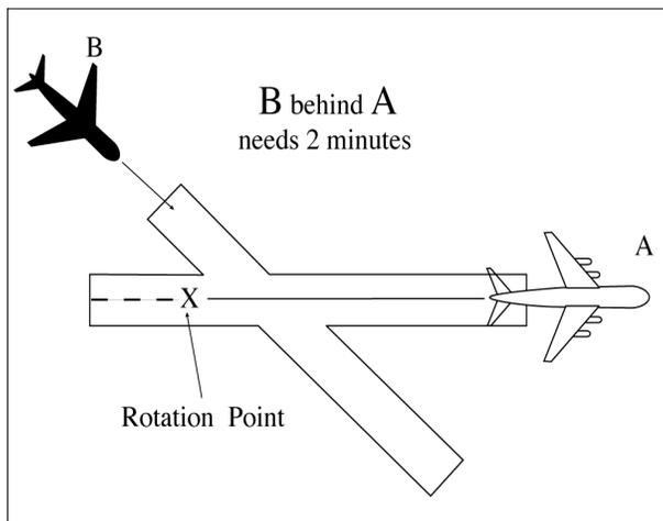
1. All aircraft landing on a crossing runway behind a departing super or heavy, or a small aircraft landing on a crossing runway behind a departing B757, if the arrival flight path will cross the takeoff path behind the departing aircraft rotation point. (See FIG 3-10-11.)
