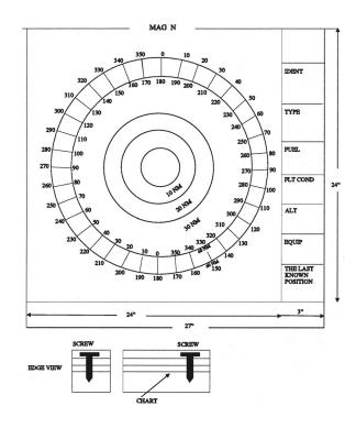
Maintain an aircraft orientation plotting board (see FIG 16–1–1), parallel rulers, plotters, and fine–line china marking pencils for use in aircraft orientation. Record pertinent information directly on the board using the marking pencils. After the orientation is
