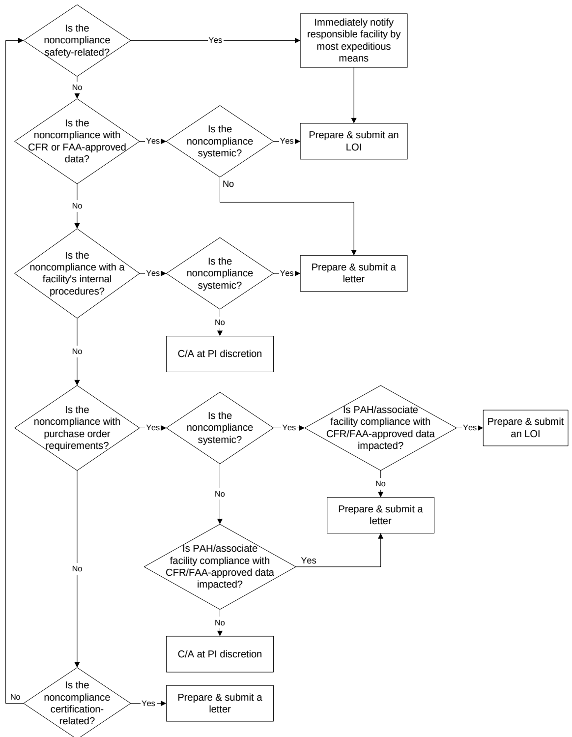
FIGURE 22. CORRECTIVE ACTION FLOWCHART
