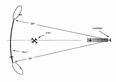
The pattern is used for localizer width checks. It is flown 90° to the localizer centerline with approximately 5 mile legs each side. Distance from the Localizer antenna is between 4 and 18 miles (normally 10 nm) from the Localizer antenna.
