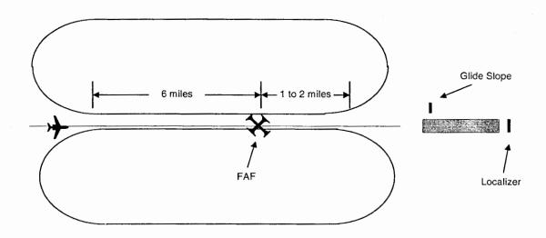
The flight inspection holding pattern is flown on centerline from 6 miles outside the Final Approach Fix (FAF) (approximately 10 miles from the runway) to approximately 2 miles inside the FAF. The altitude will normally be at GSI corrected to true altitude. Left or right turns are at the discretion of Air Traffic. Altitude assignments can provide for departure/ arrival tunneling. Aircraft may be vectored on outbound legs.
