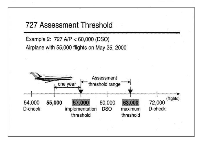
This example is for a 727 airplane with 55,000 flight cycles on May 25, 2000. This was over 45,000 flights (75% DSG/DSO), but less than 60,000 flights (DSG/DSO); thus:
