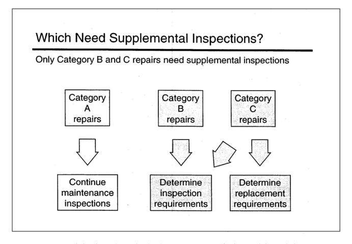
Once a repair has been determined to be Category A, no further work is needed. It can continue to be inspected by normal maintenance.
