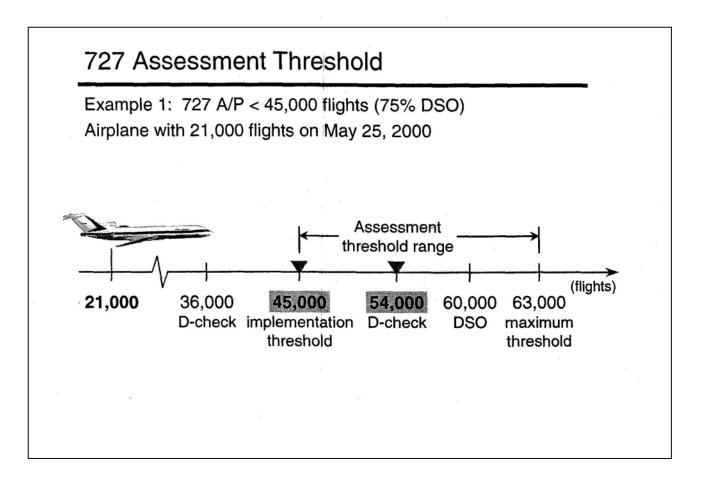
This example is of the implementation and assessment thresholds for a 727 airplane that had 21,000 flight cycles on May 25, 2000. This was less than 45,000 flights (75% DSG/DSO); thus:
