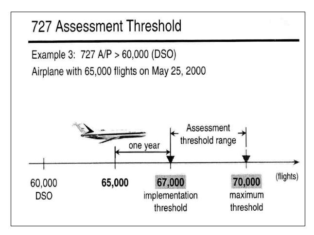
This is an example for a 727 airplane with 65,000 flight cycles on May 25, 2000. The aircraft was over 60,000 flights (DSG/DSO); thus:
