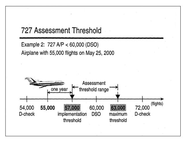
This example is for a 727 airplane with 55,000 flight cycles on May 25, 2000. This was over 45,000 flights (75 percent DSG/DSO), but less than 60,000 flights (DSG/DSO); thus:
