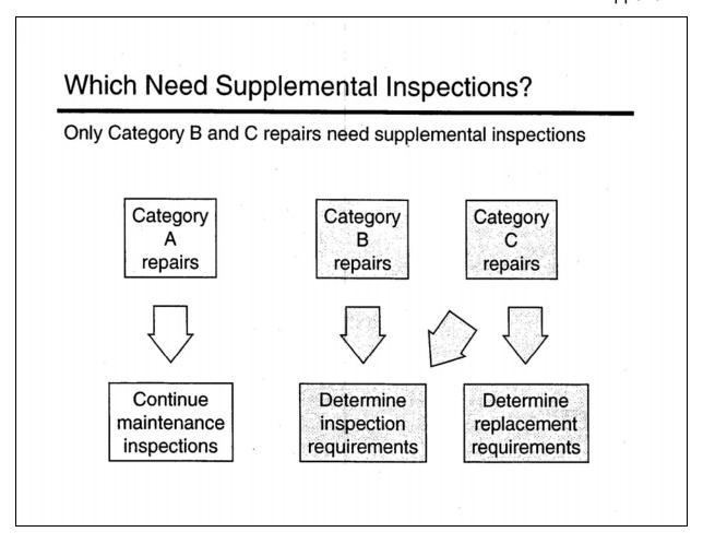
Once a repair has been determined to be Category A, no further work is needed. It can continue to be inspected by normal maintenance.
