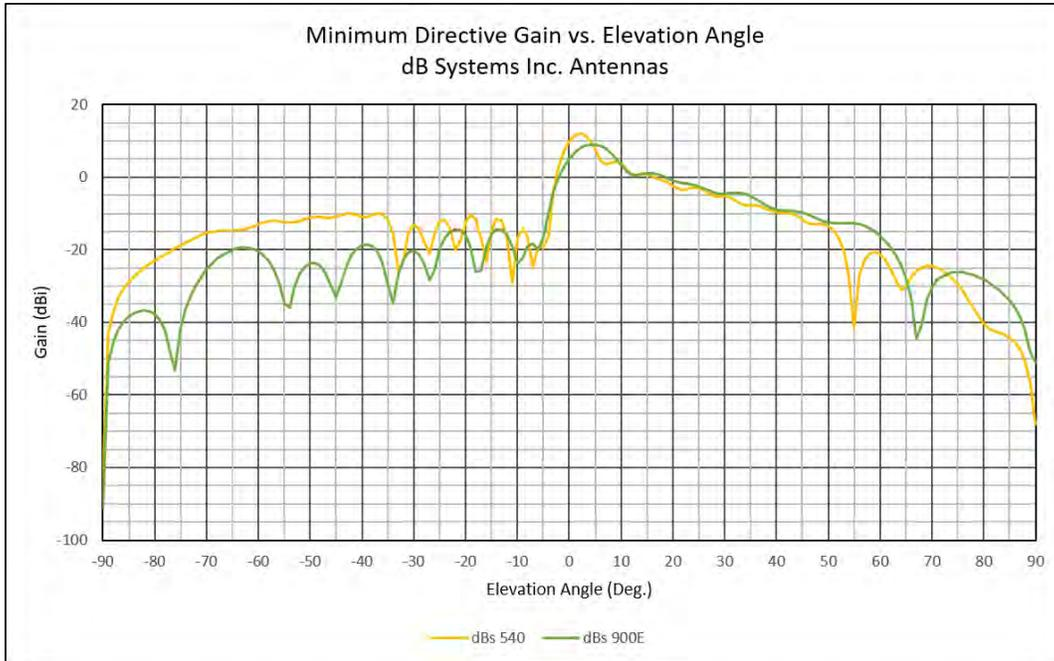
**Figure 4-15. dB Systems, Inc. DME Antennas Minimum Directive Gain for 540 and 900E Models**
