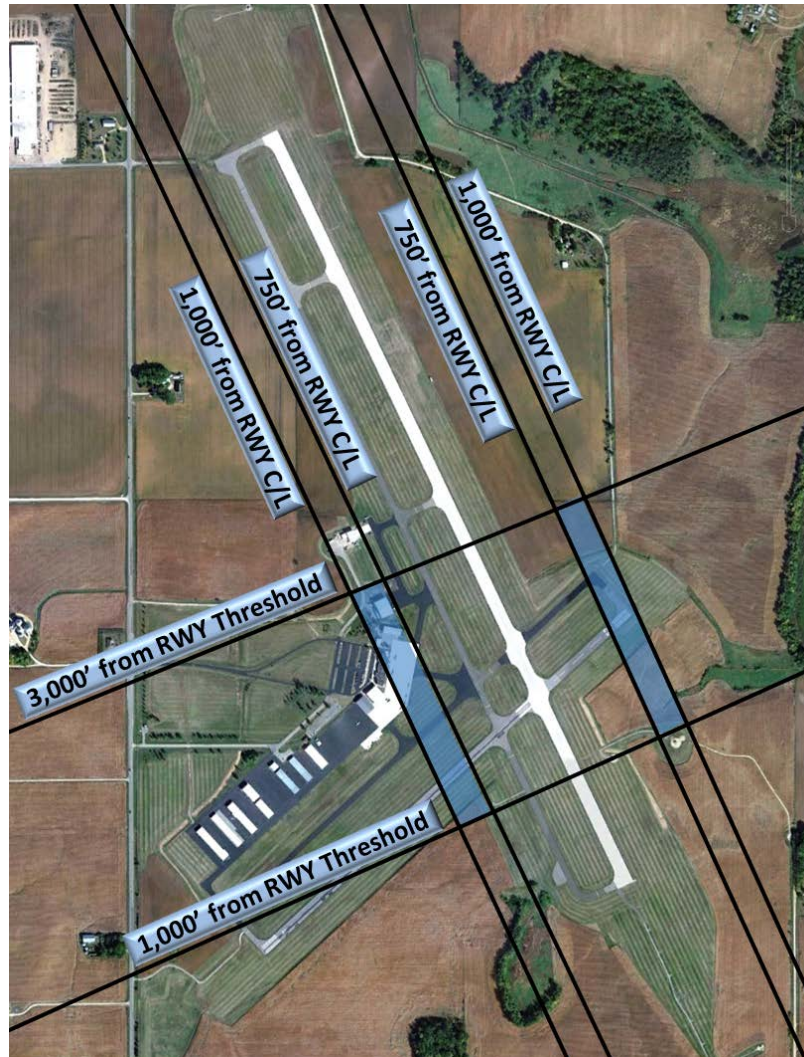
Figure 3-2. Siting Criteria for Airports with Precision Runways without RVR
