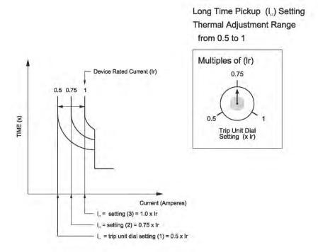
Figure H-3. Thermal-Magnetic Device with Adjustable Instantaneous Pick-up Setting
