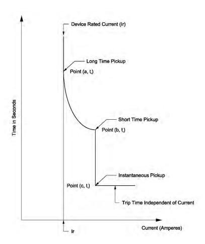
Figure H-1. Typical Thermal Magnetic Device Trip Unit TCC
