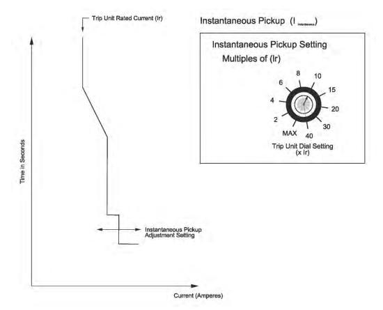
Figure H-9. Electronic Trip Unit, Instantaneous Pickup Adjustment Setting
