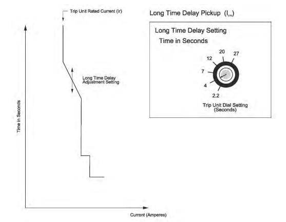
Figure H-6. Electronic Trip Unit, Long-Time Delay Adjustment Setting
