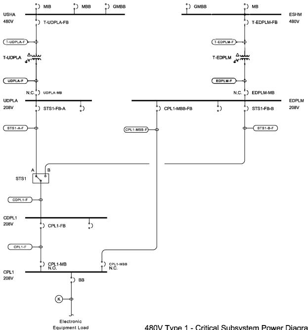
480V Type 1 - Critical Subsystem Power Diagram
