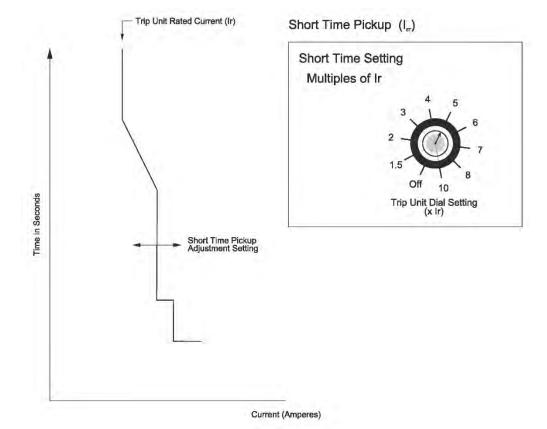
Figure H-7. Electronic Trip Unit, Short-Time Pickup Adjustment Setting
