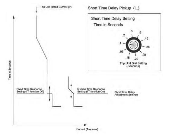
Figure H-8. Electronic Trip Unit, Short-Time Delay Adjustment Settings
