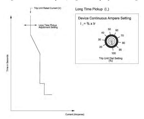
Figure H-5. Electronic Trip Unit, Long-Time Pickup Adjustment Setting
