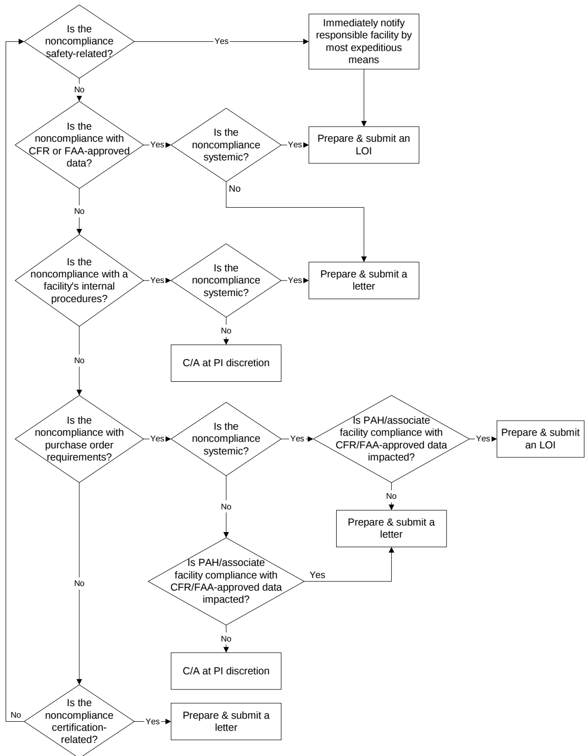
FIGURE 16. CORRECTIVE ACTION FLOWCHART
