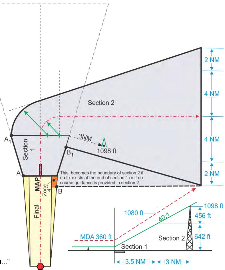
c. Evaluate the 40:1 surface from the MAP to the clearance limit (end of the missed approach segment). If obstacles penetrate the surface, take action to eliminate the penetration.
