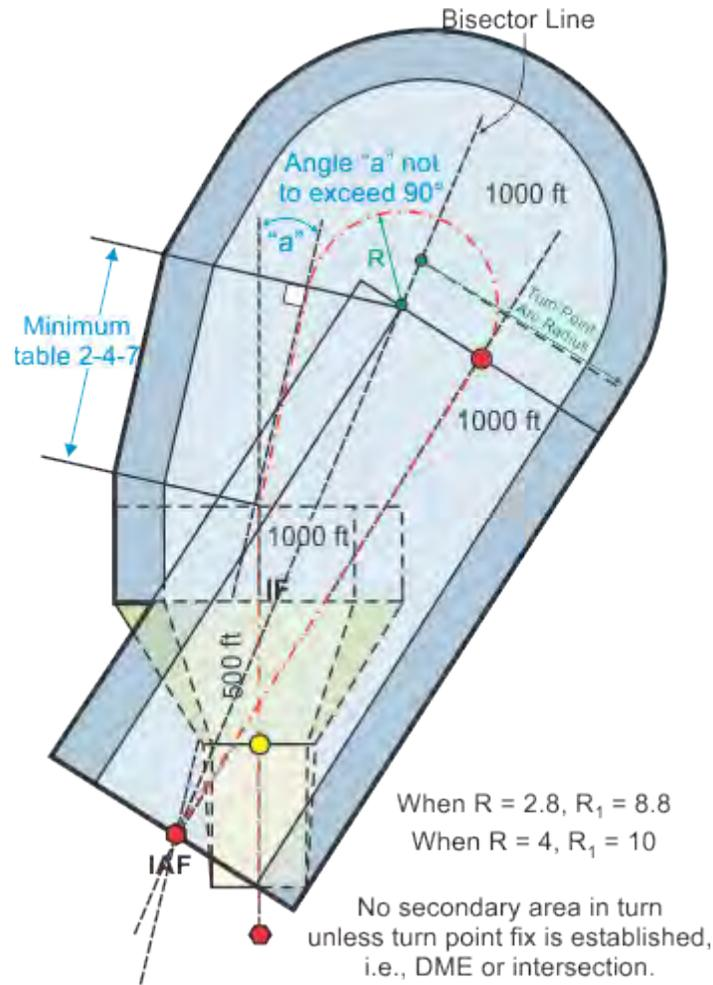
**Table 2-4-7. Minimum Distance from Roll Out Point to Point of Intersection**
