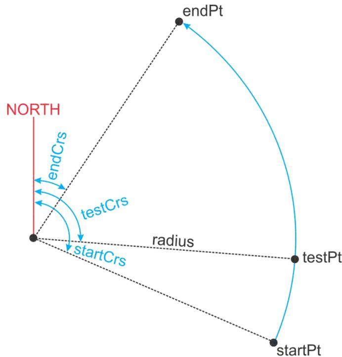
(1) *Step 1.* Use inverse algorithm to calculate distance and azimuth from center to testPt. Denote values as *dist* and *crs*, respectively.
