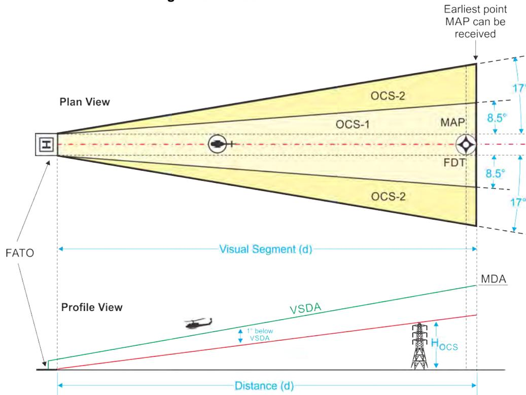
(1) *Step 1.* Calculate OCS-1 width ( $W_{OCS-1}$ ) at distance ( $d$ ) from the FATO edge using formula G-2.
