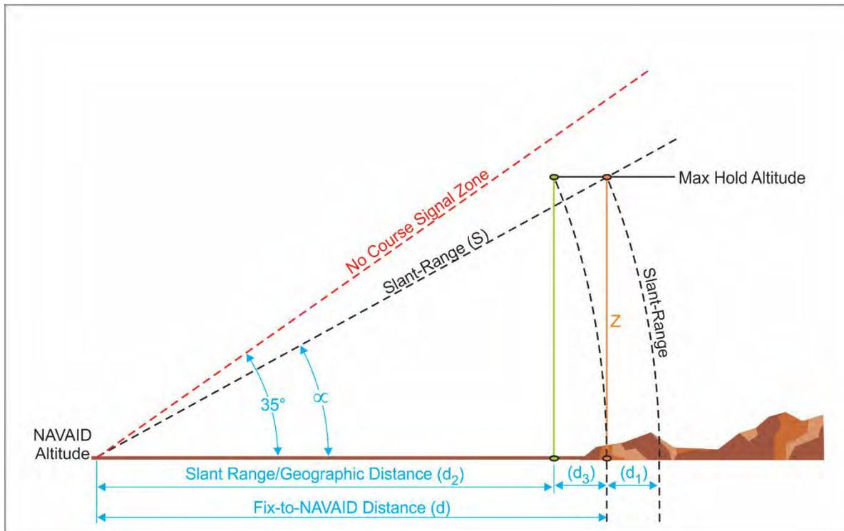
a. Formula 16-14-1 is used to determine the height above the NAVAID at the maximum holding altitude, and converted to NM for use in other calculations.
