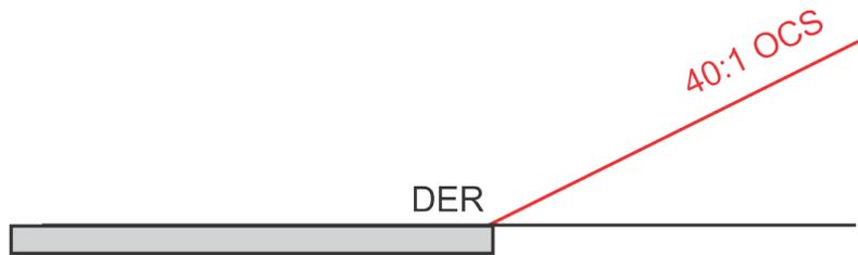
**a.** Low, close-in OCS penetrations. Do not publish a CG to a height of 200 feet (400 feet for helicopters) or less above the OCS start elevation.
