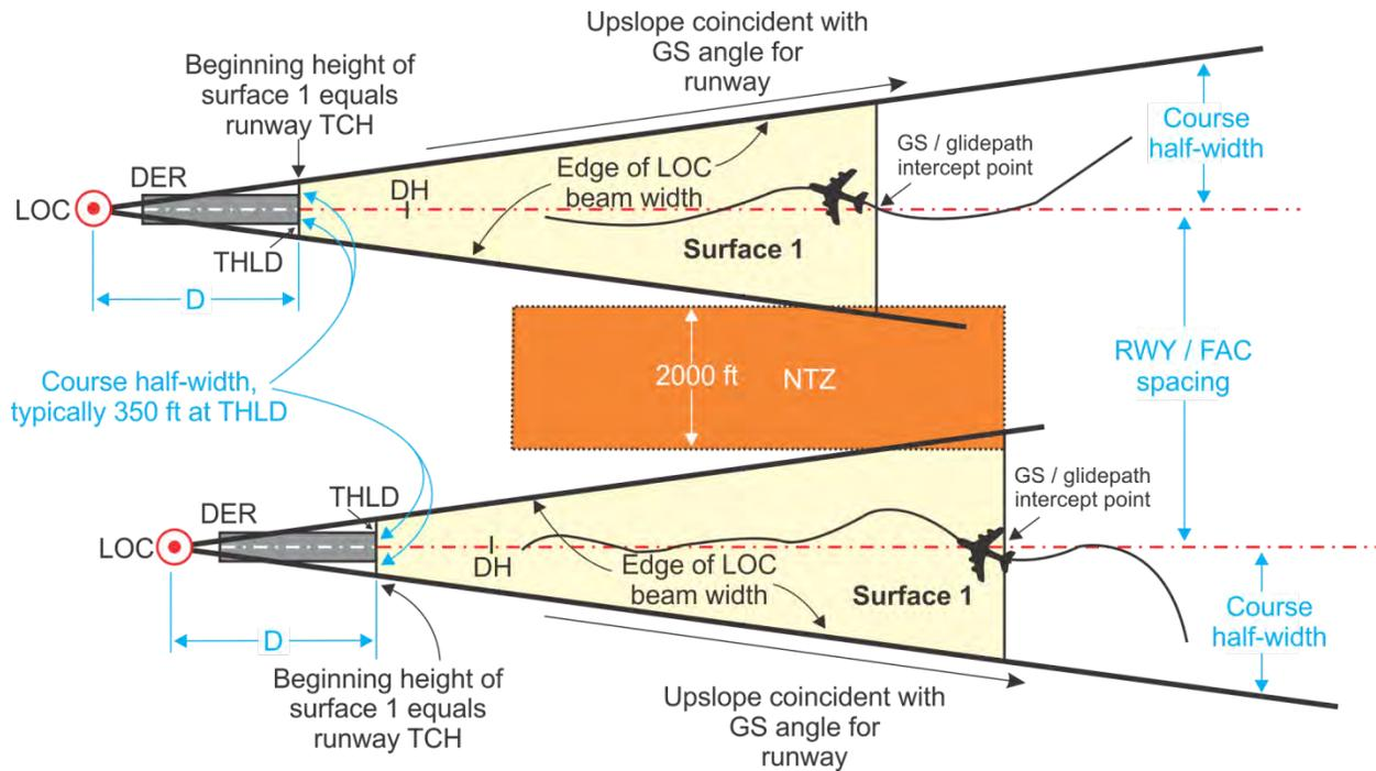
(1) Length. Surface 1 begins over the runway threshold at a height equal to the TCH for the runway, and continues outward and upward at a slope that is coincident with the glide slope/glidepath, to its ending at the GS/vertical path intercept point.
