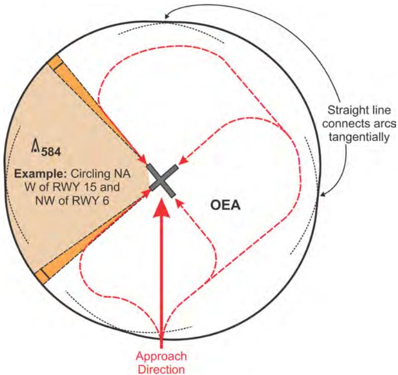
**Figure 2-7-5. Complex Restricted Circling Area, Straight-in Aligned Approach (<180 Degrees, Intersecting Runways)**
