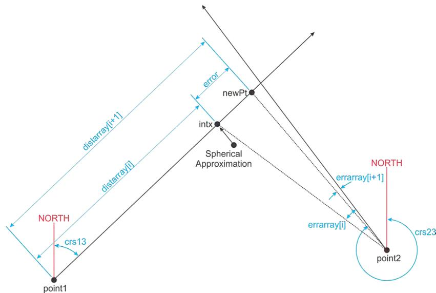
(1) *Step 1.* Use inverse algorithm to calculate distance, azimuth, and reverse azimuth from pt1 to pt2. Denote these values by dist12, crs21 and crs12, respectively. Run a check to see if pt1 lies on the geodesic defined by pt2 and crs23 and if pt2 lies on the geodesic defined by pt1 and crs13:
