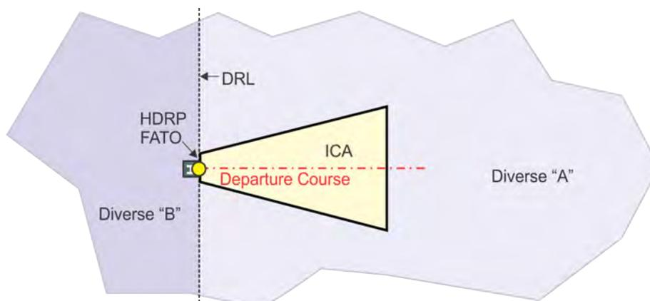
(1) ICA. Apply paragraph 13-1-7 to evaluate the ICA using a 40:1 OCS slope (see figure 13-2-1).
