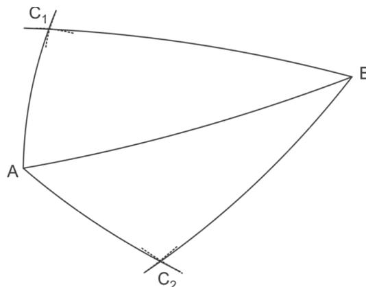
(1) *Step 1.* Run Inverse to find length and bearings between A and B. Use spherical triangles to find angles  $A = BAC_1 = BAC_2$ ,  $B = ABC_1 = ABC_2$ , and  $C = BC_1A = BC_2A$ :
