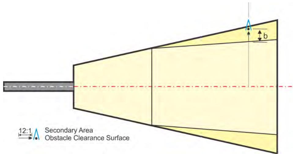
**13-1-5. CGs.** DP obstacle clearance is based on a minimum CG performance of 200 ft/NM [(400 ft/NM for helicopters), see figure 13-1-3].
