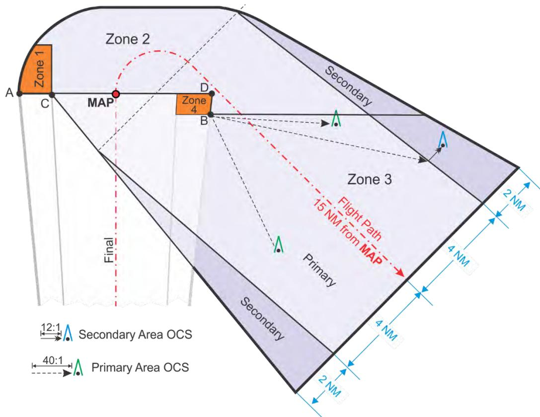
**c.** Secondary area. In the secondary area no obstacles may penetrate a 12:1 slope which extends outward and upward from the 40:1 surface from the inner to the outer boundary lines of the secondary area.
