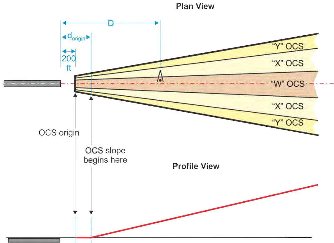
c. Obstacle effective elevation ( $O_{EE}$ ). Because the earth curves away from the OCS as distance from course centerline increases, the MSL elevation of an obstacle is reduced to account for this. Use formula 10-2-3 to calculate  $O_{EE}$ .
