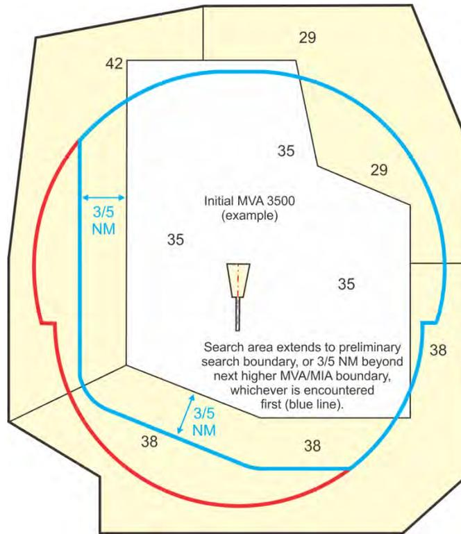
Figure 13-5-8. Permitted DVA Headings Based on Obstacles
