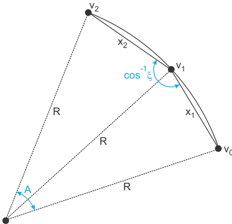
(1) *Step 1.* Set initial number of sub-arcs to use. The fixed value  $n = 16$  has been found through trial-and-error to be a good starting value. Alternatively, the initial value of  $n$  may be calculated based on the arc's subtended angle and its radius (i.e., its approximate arc length).
