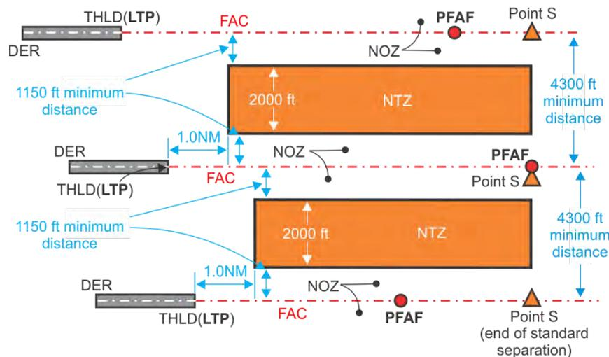
**Note:** For triple approaches, the highest glide slope intercept altitude should be associated with the approach to the center runway and that intercept point establishes where point S is located for the other two runways.
