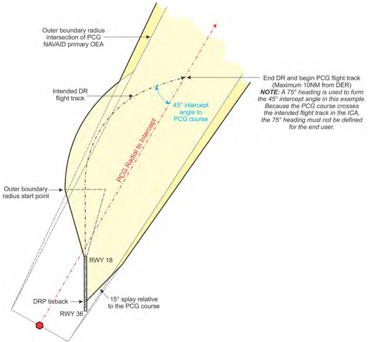
Figure 13-3-10. Turn to Intercept Radial with Arc Extension (Off Airport NAVAID)
