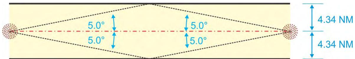
**Figure 14-5-2. LF Segment Secondary Obstacle Clearance Area**
