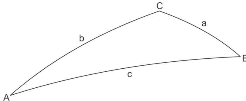
(1) *Step 1.* Run Inverse to find arc length from A to B and bearings A to B and B to A. Compute differences of bearings to find angles A and B of the spherical triangle ABC. More than one valid solution may result. Choose the solution closest to the original points.
