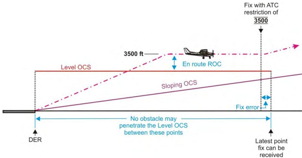
(2) Where the height of the level OCS is less than the height of the sloping OCS, apply a 30.38:1 sloping OCS into the next segment from the primary area boundary of the level OEA. The 30.38:1 OCS originates at the same height as the level OCS. Penetrations may not be mitigated by a CG; if penetrations exist, the maximum altitude authorized at the fix with the altitude restriction must be increased until the penetration is eliminated (see figure 13-6-5).
