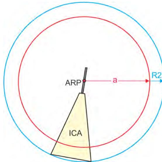
a = radius used to establish VCA via Formula 13-4-1. This example used 1,000 feet MSL and 200 KIAS to establish the VCA.
