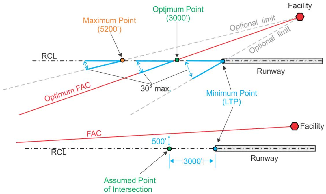
**Figure 4-2-2. Alignment Options for Final Approach Course, On-Airport VOR, No PFAF, Circling Approach Procedure**
