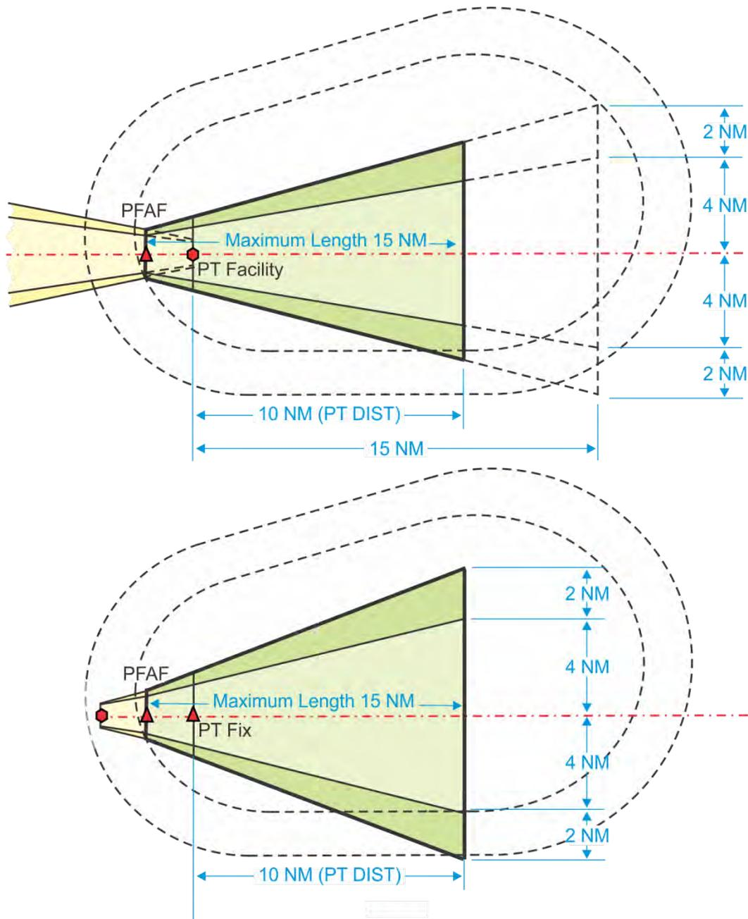
**Figure 2-5-7. Intermediate Area Within PT Area, PT Facility/Fix Used as a Stepdown Fix**
