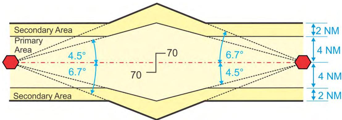
**c.** Offset COP. If the changeover point is offset due to facility performance problems, the system accuracy lines must be carried from the farthest facility to a position abeam the changeover point, and these lines on each side of the airway or route segment at the COP are joined by lines drawn directly from the nearer facility. In this case the angles of the lines drawn from the nearer facility have no specific angle (see figure 14-1-13).
