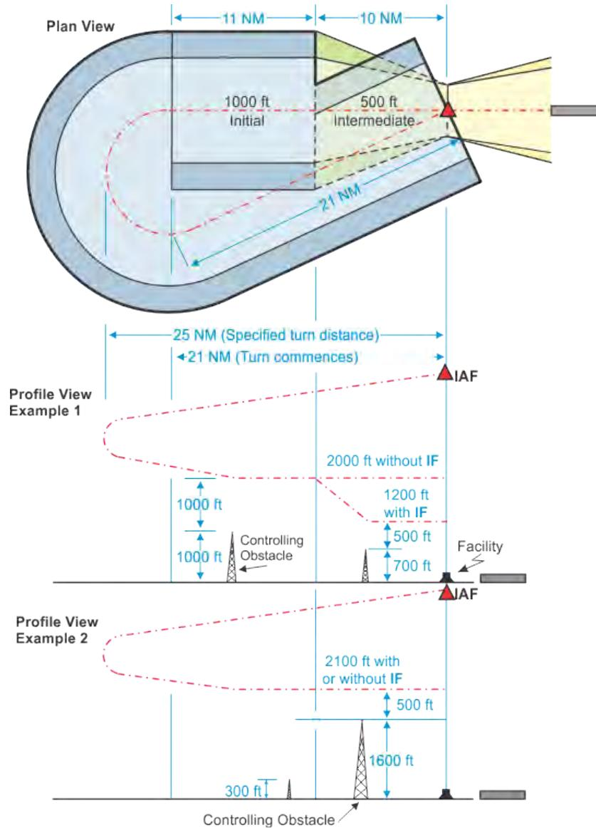
**d.** Descent gradient. The optimum descent gradient is 800 ft/NM. The maximum gradient is 1000 ft/NM.
