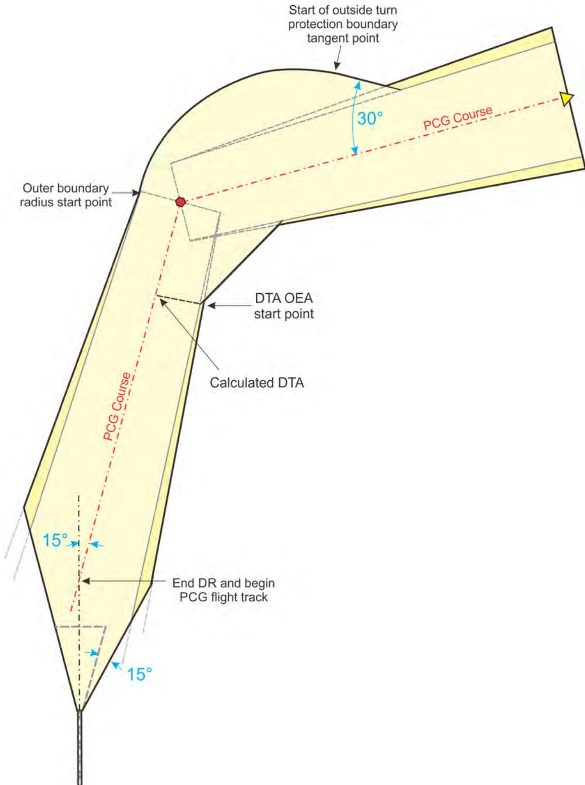
**13-3-5. Routed Departure Obstacle Evaluation.** Obstacles must not penetrate the OCS. Evaluate obstacle against the OCS along the routed DP using either a 40:1 or 12:1 slope until the terminal portion of the DP ends (see figure 13-3-20 through figure 13-3-22, formula 13-1-1 and formula 13-1-2).
