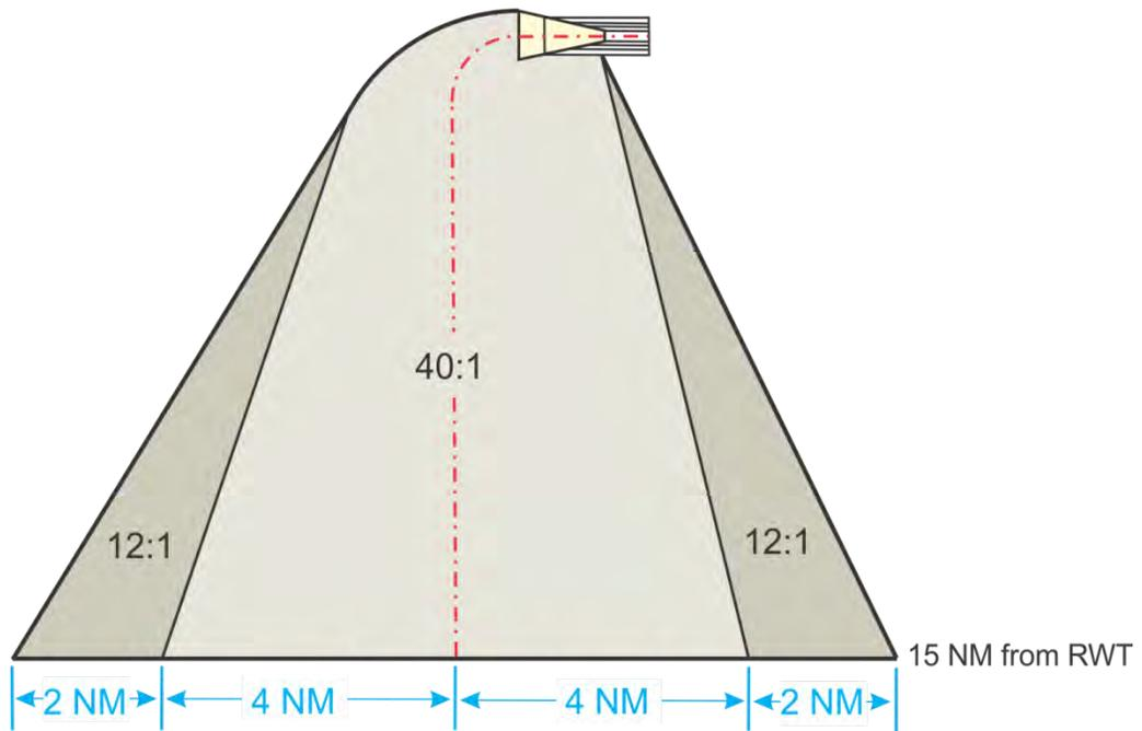
Figure 10-5-5. Turning Missed Approach OCS Detail
