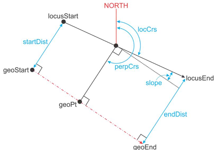
(1) *Step 1.* Use section 3 algorithm 9 to determine whether testPt lies on loc. This same step will return a reference to the projection of testPt onto the defining geodesic. Denote this reference as geoPt.
