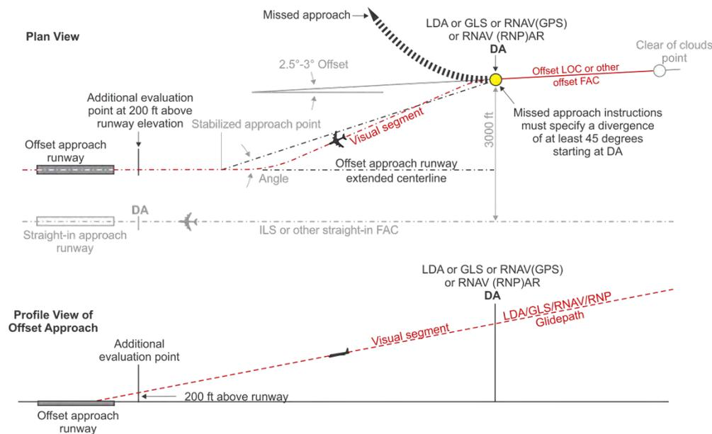
**b. Offset FAC Approach.** Missed approach procedures for SOIA offset FAC approaches must specify a turn to a heading at the MAP (the DA). Use the current TERPS evaluation for the offset FAC type of approach navigation with a turning missed approach.
