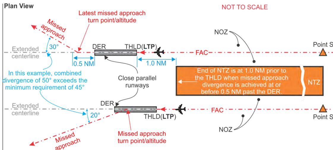
**Figure 15-2-2. Missed Approach Divergence Delayed Beyond 0.5 NM**
