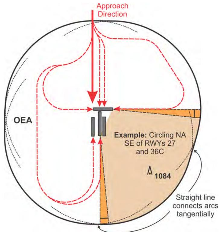
**Figure 2-7-7. Complex Restricted Circling Area, Expanded Restricted Area, Straight-in Aligned Approach**
