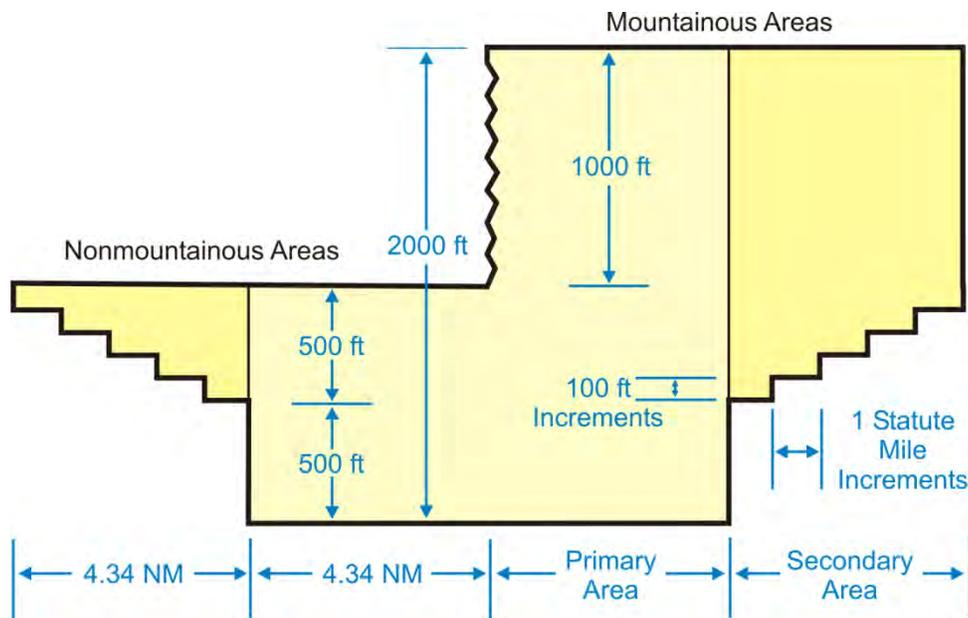
(b) Beyond the 25-NM distance from the facility, the secondary obstacle clearance plane is flat. This plane is drawn from the primary area boundary 500 feet above the obstacle which dictates its MOCA and extending to the edge of the secondary area. If an obstacle penetrates this surface the MOCA for the segment will be increased so as to provide 500 feet of clearance over the obstacle (see Figure 14-5-4 and paragraph 14-5-1.d(2)(c)).
