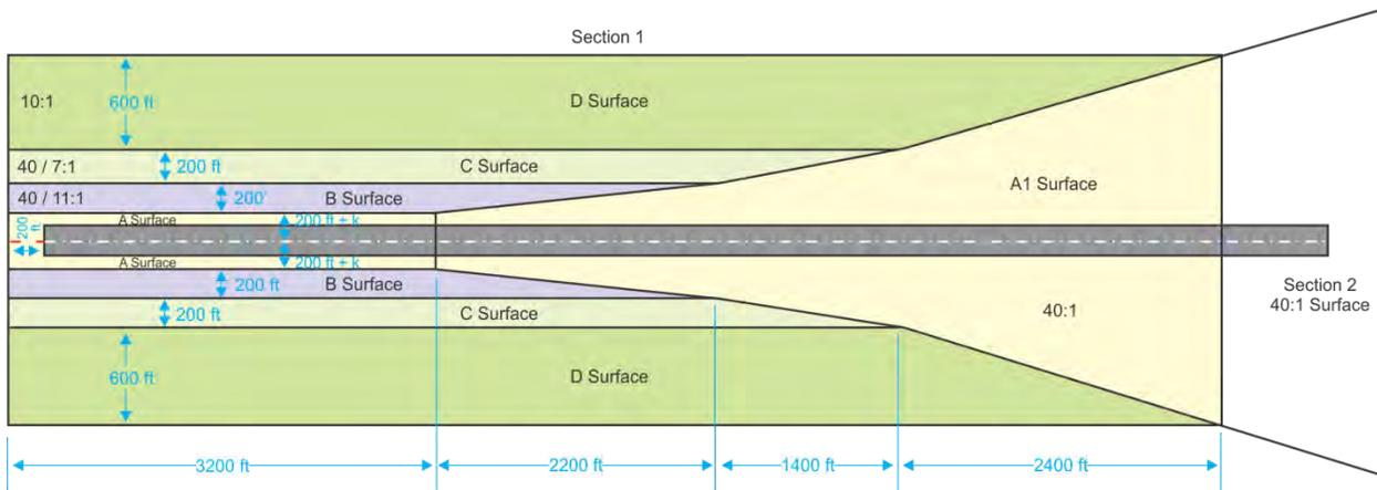
(2) The OCS slopes associated with surface A, B, C, and D are depicted in figure 10-5-2. Surface A1 has a slope of 40:1 rising in the direction of the missed approach.
