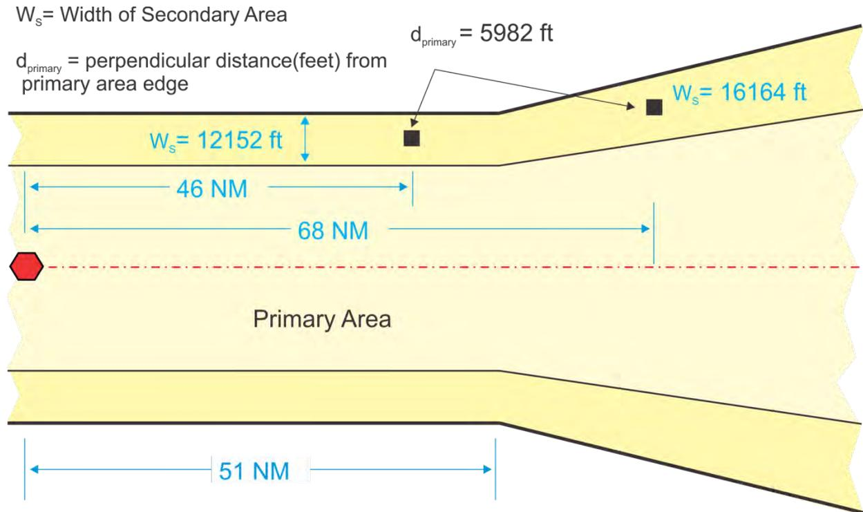
**Example:** An obstacle which reaches 1875 feet MSL is found in the secondary area; 5982 feet from the primary area edge, and 46 NM from the facility (see figure 14-2-1 and figure 14-2-2).
