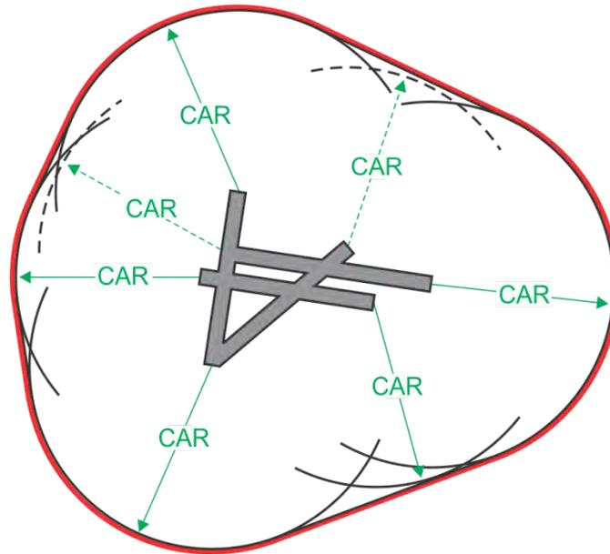
**b. Obstacle clearance.** The minimum ROC in the circling approach OEA is 300 feet. Adjustments must be applied as specified in paragraph 3-2-2.c.
