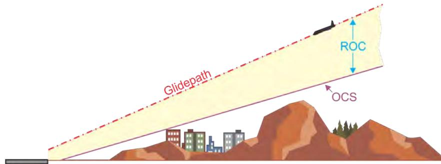
(1) If the OCS is penetrated, the OCS slope may be adjusted upward, thereby increasing the glidepath angle. The glidepath angle would increase because it is dependent on the required slope.
