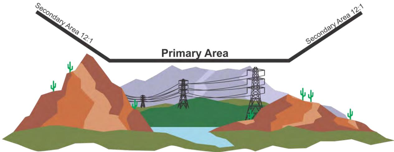
**2-8-6. Turning Missed Approach Area.** If a turn of more than 15 degrees from the FAC is required, a turning or combination straight and turning missed approach area must be constructed. If the HAT or HAA value associated with the DA/MDA/CMDA is less than 400 feet, construct a combination straight and turning missed approach (see paragraph 2-8-8). The minimum turn altitude is 400 feet above touchdown zone elevation (TDZE)/airport elevation, rounded to the nearest foot increment.
