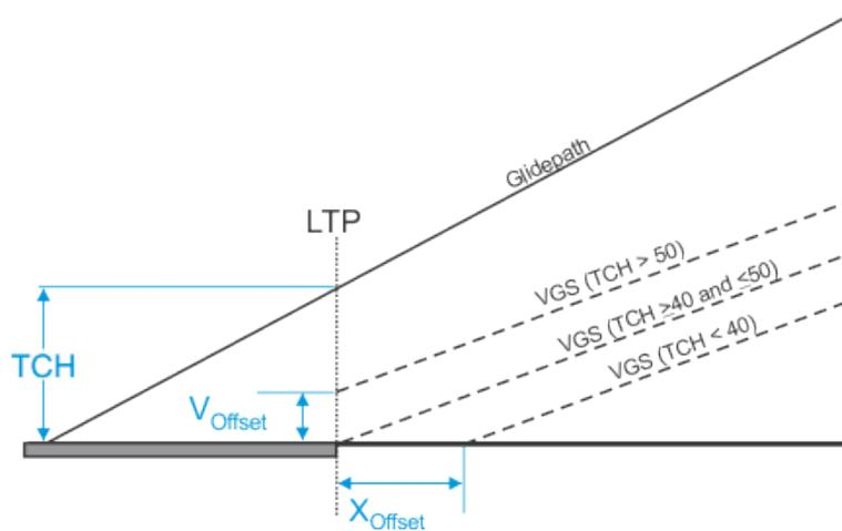
f. VGS slope elevation. The VGS slope is based on  $\frac{2}{3} \times \text{GPA}$ . Apply formula 2-6-12 to determine the VGS elevation.
