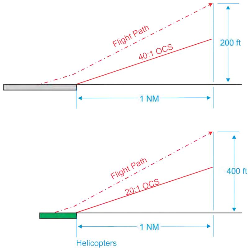
**a.** Calculating CGs to clear obstacles. CGs in excess of 500 ft/NM (600 ft/NM for helicopters) require approval (see paragraph 1-4-2). Calculate CGs using formula 13-1-3.
