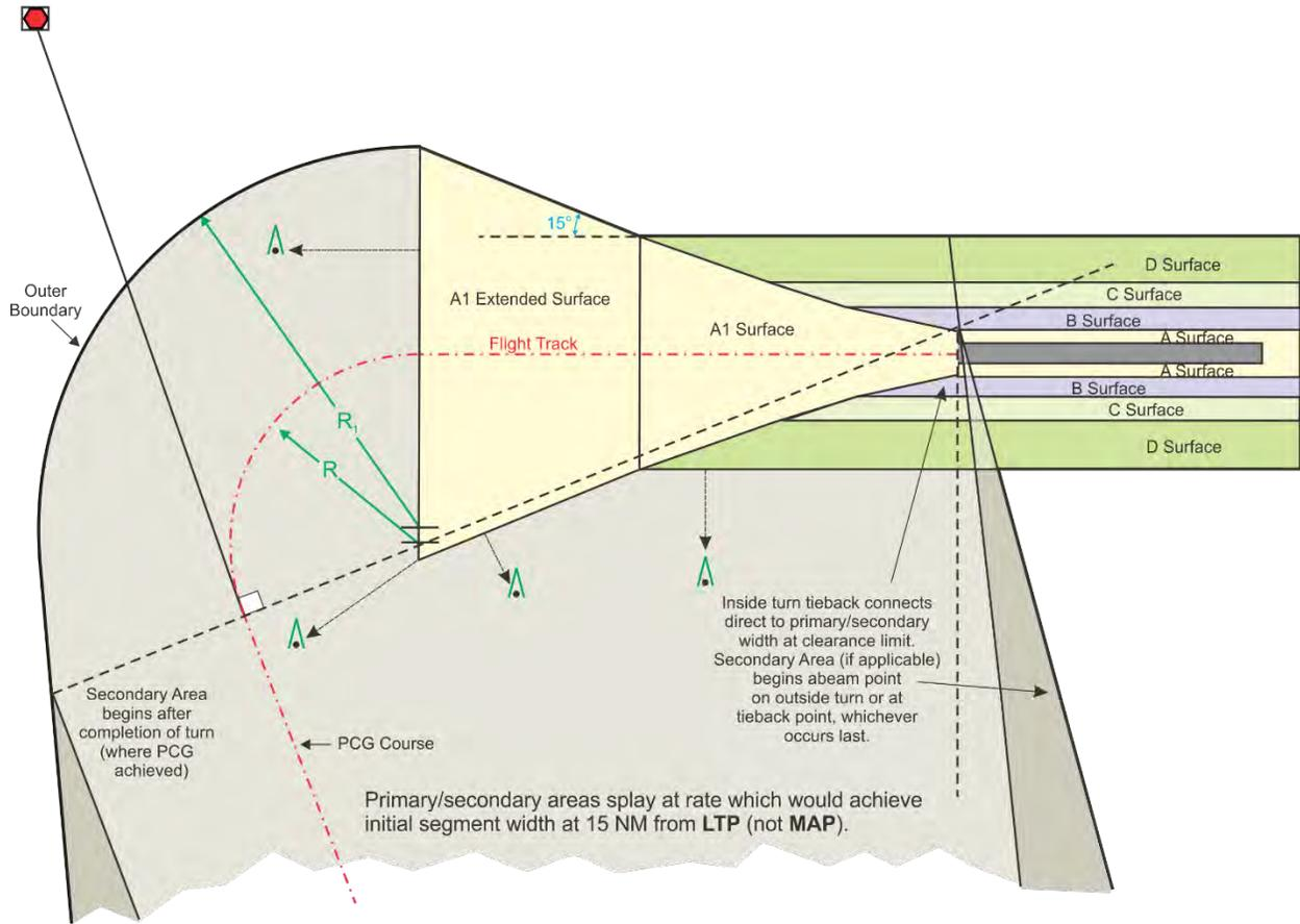
**Figure 10-5-6. Turning Missed Approach OCS Detail (Continued)**
