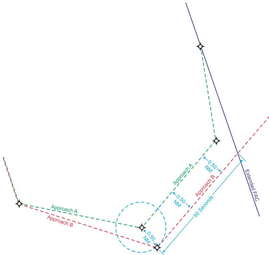
**Figure 15-5-2. Incorrect Flight Procedure Selection (RF Legs)**
