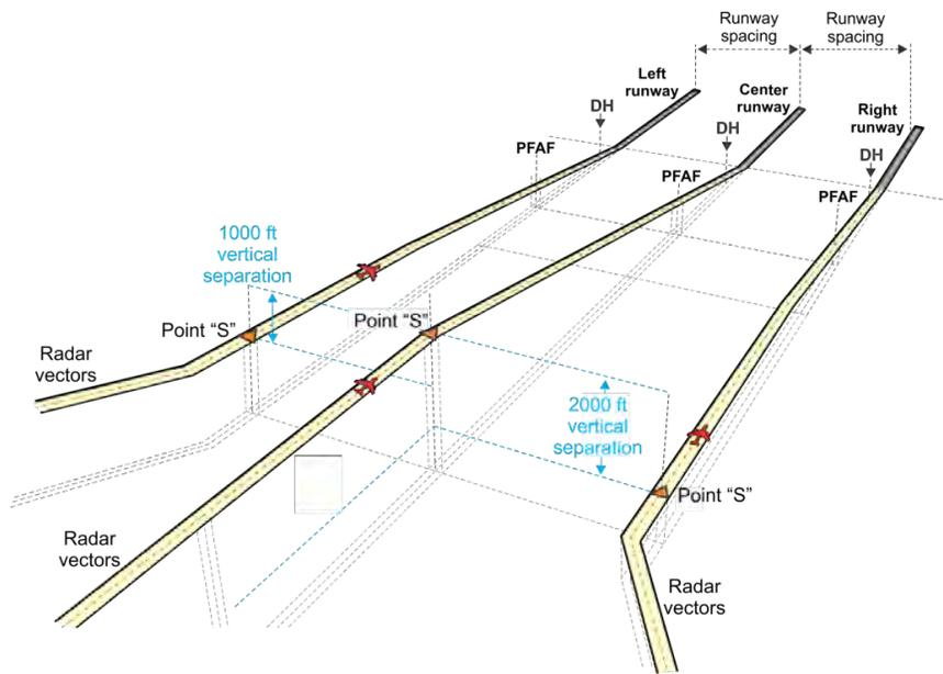
**Figure E-3. Example of PBN Simultaneous Independent Procedures Considered Established on Approach Dual Approaches**
