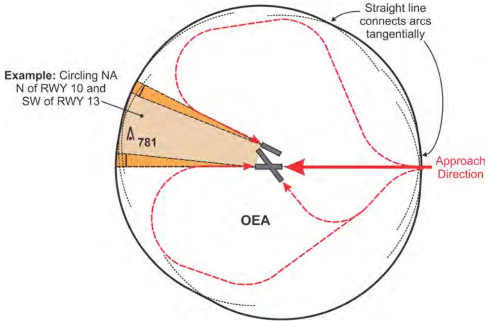
**Figure 2-7-6. Complex Restricted Circling Area, Straight-in Aligned Approach (<180 Degrees, Parallel Runways)**
