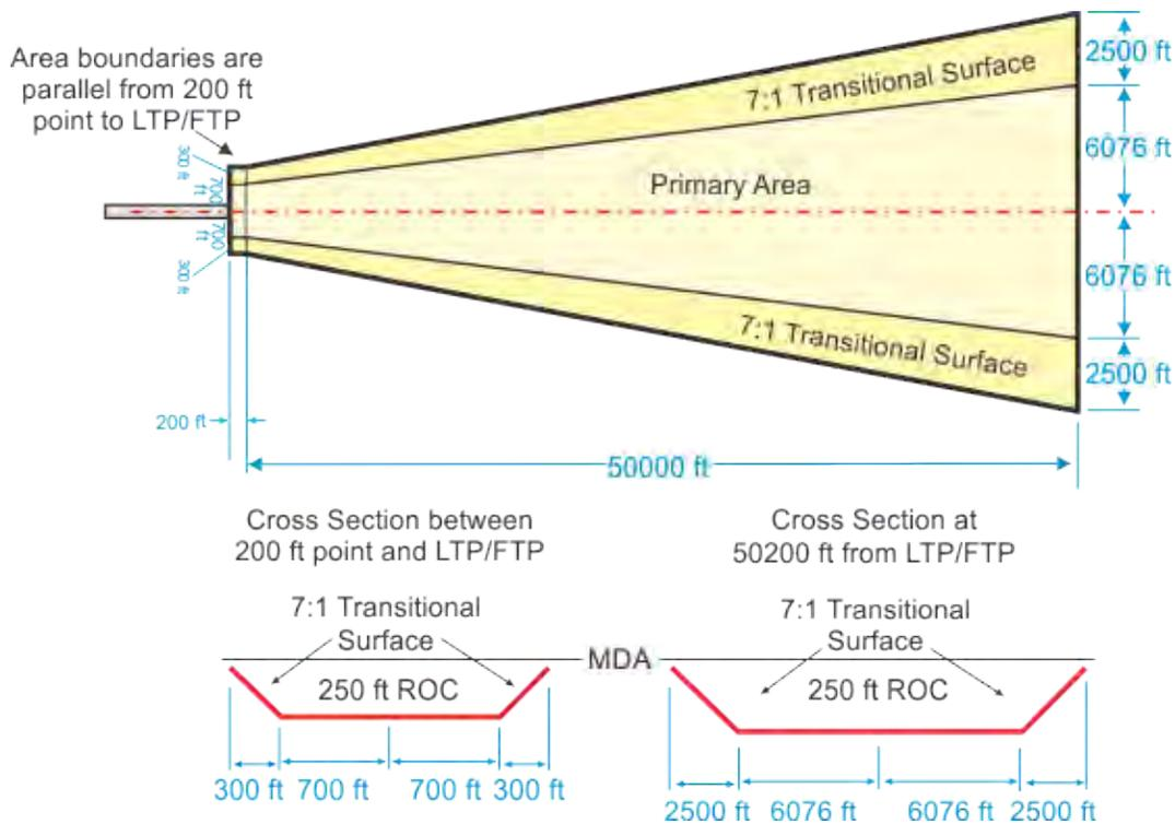
**8-1-4. Obstacle Clearance.** The minimum ROC in the final approach area is 250 feet plus adjustments as specified in paragraph 3-2-2. In addition, the MDA established for the final approach area must assure that no obstacles penetrate the 7:1 transitional surfaces.
