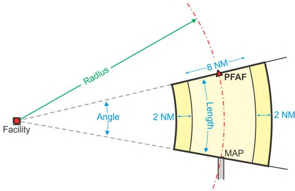
(3) Obstacle clearance. The minimum obstacle clearance in the primary area is 500 feet. The ROC in the secondary area is 500 feet at the primary boundary, tapering uniformly to zero feet at the outer edge (see figure 5-3-3). The minimum ROC at any given point in the secondary area is determined by formula 5-3-2. Adjustments must be applied as specified in paragraph 3-2-2.
