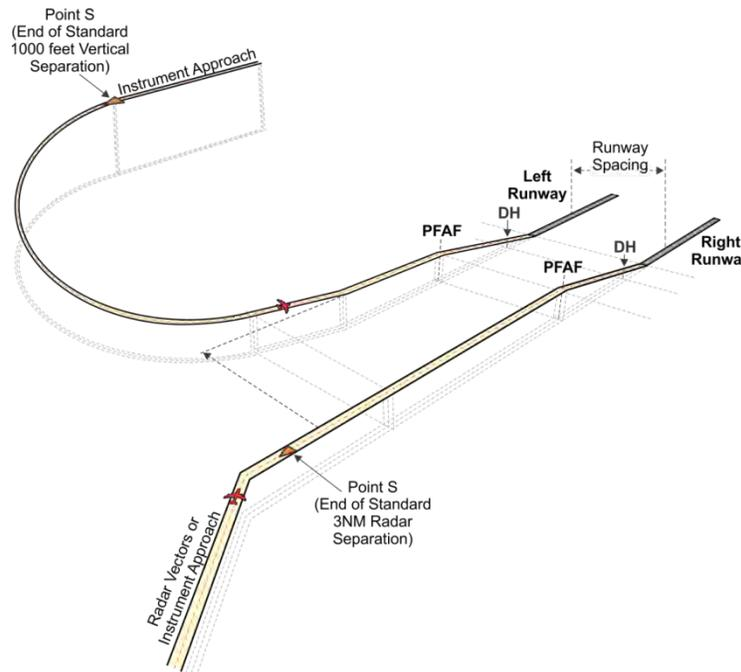
**3. Overview.** Simultaneous independent approach operations use reduced air traffic separation and provide a means to maintain near-optimum airport efficiencies in conditions of reduced ceiling and visibilities. A procedure is authorized (by applicable chart notes) if it meets the guidance in this order and other applicable 8260-series criteria and ATC guidance.
