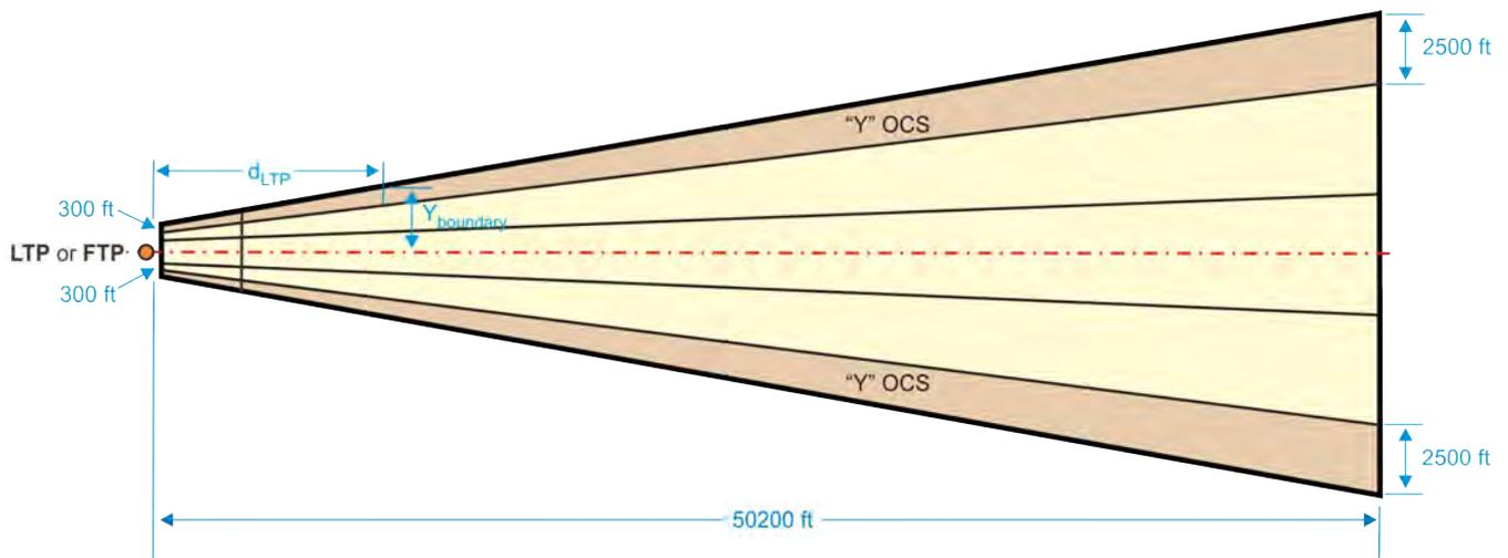
**a.** Width. Use formula 10-2-9 to calculate the perpendicular distance ( $Y_{boundary}$ ) from the course to the outer boundary of the "Y" OCS at a specified distance.
