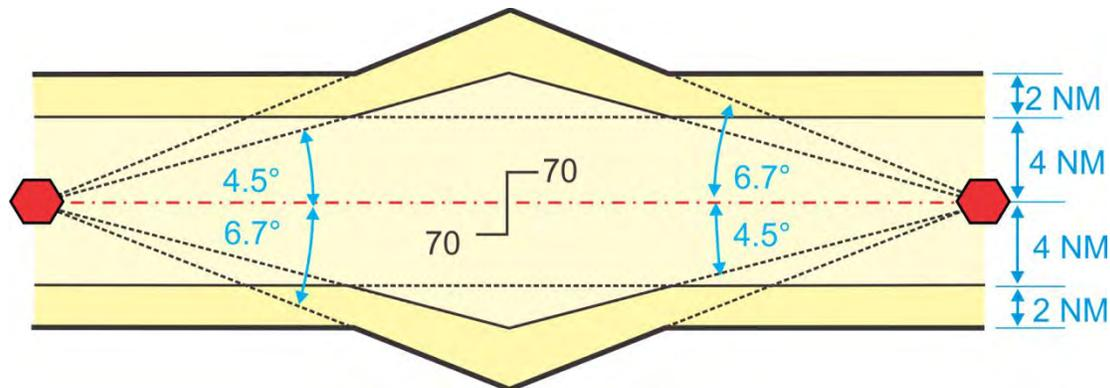
c. Termination point. Where the airway or route terminates at a facility or radio fix the boundaries are connected by an arc in the same way as those in the primary area. Figure 14-1-8 and its inset shows termination point secondary areas.
