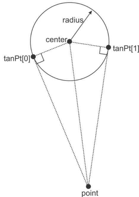
(1) *Step 1.* Use the inverse algorithm to calculate the distance, azimuth, and reverse azimuth from point to center. Denote these values by  $crsToCenter$ ,  $crsFromCenter$ , and  $distToCenter$ , respectively.
