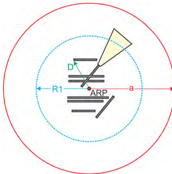
a = radius used to establish VCA via Formula 13-4-1. This example used 1,000 feet MSL and 250 KIAS to establish the VCA.
