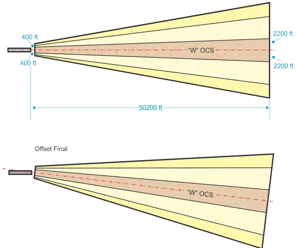
**a. Width.** The width is 400 feet on each side of course at the beginning, and expands uniformly to 2200 feet on each side of course at 50200 feet from LTP/FTP. Use formula 10-2-4 to calculate the "W" OCS half-width at a specified distance.
