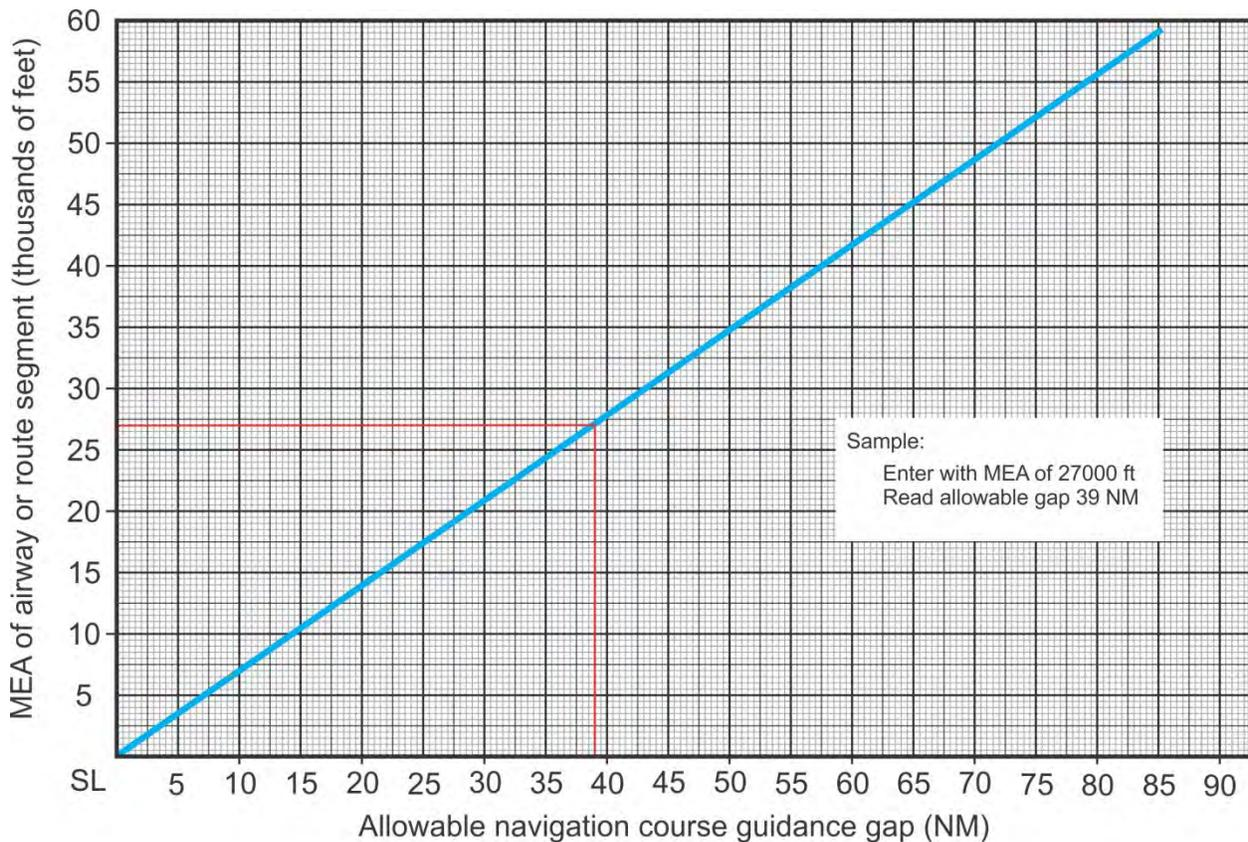
**Example:** The problem drawn on the chart shows the method used to determine the allowable gap on a route segment with a proposed MEA of 27000 feet. Enter the graph at the left edge with the MEA of 27000 feet. Move to the right to the interception of the diagonal line. Move to the bottom of the graph to read the allowable gap. In the problem drawn, a 39-NM gap is allowable.
