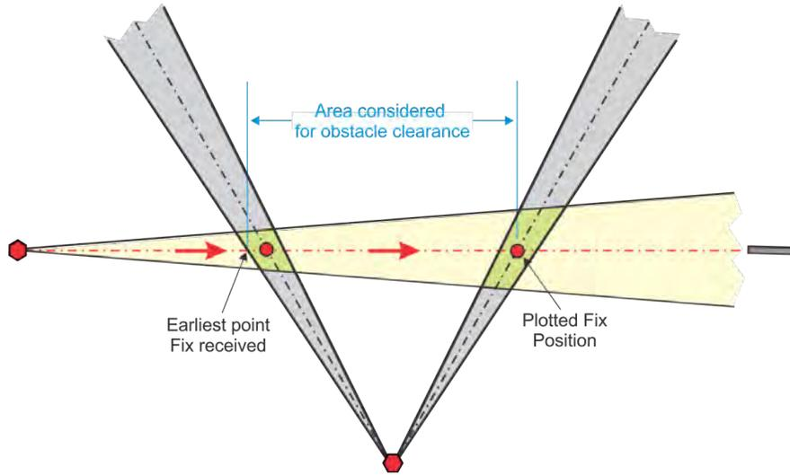
**Figure 2-9-8. Construction of Fix Displacement Area for Obstacle Clearance**
