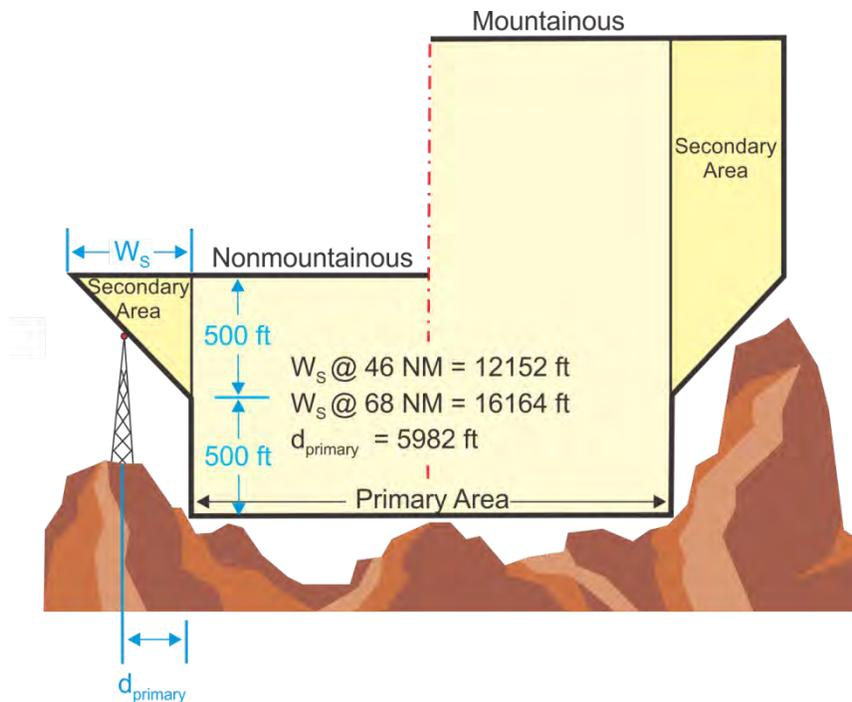
**Figure 14-2-2. Plan View, Secondary Area Obstacle Clearances**
