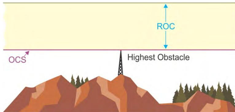
**2-1-4. Sloping OCS.** The method of applying ROC, in segments dedicated to descending on a glidepath or climbing in a departure or missed approach segment, requires a different obstacle clearance concept than the level OCS because the ROC value must vary throughout the segment. The value of ROC near the runway is relatively small and increases throughout the segment.
