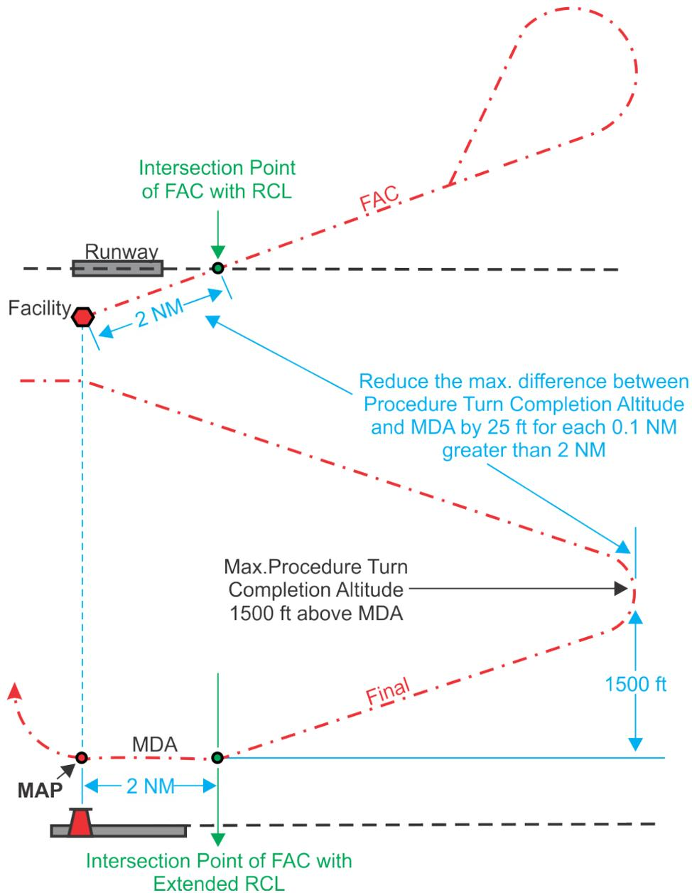
Figure 4-2-6. PT Altitude, Circling
