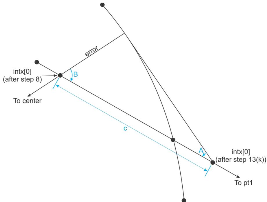
(1) *Step 1.* Use section 4 algorithm 1 to find the perpendicular projection point from arc center point (center) to the geodesic defined by starting point pt1 and azimuth crs1. Denote this point by perpPt. Denote the distance as perpDist.
