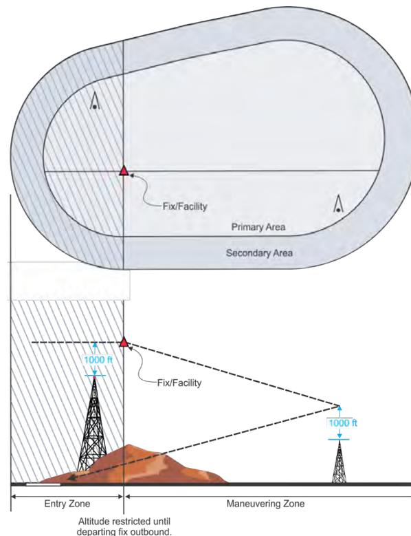
d. Descent gradient. The optimum descent gradient in the initial approach is 250 ft/NM. Where a higher descent gradient is necessary, the maximum permissible gradient is 500 ft/NM. Where a PT is established over a PFAF, the PT completion altitude should be as close as possible to the PFAF altitude. The difference between the PT completion altitude and the altitude over the PFAF must not be greater than those shown in table 2-4-5. If greater differences are required for
