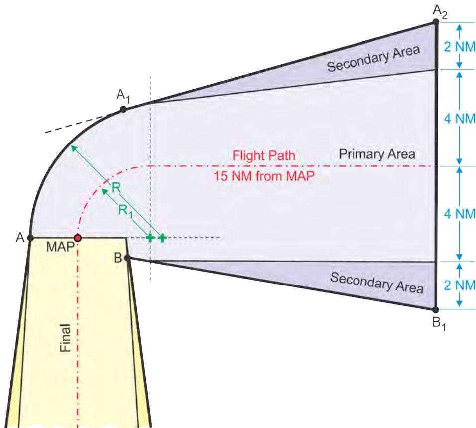
(a) Draw an arc with the radius ( $R_1$ ) from the MAP. This line is then extended outward to a point 15 NM from the MAP, measured along the line. This is the assumed flight path (see table 2-8-1).
