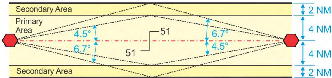
**b.** Long segments. If the distance between two facilities is over 102 NM and the COP is placed at the midpoint, the system accuracy lines extend beyond the minimum widths of 8 NM and 12 NM, and a flare results at the COP (see figure 14-1-12).
