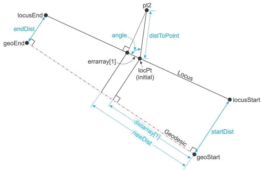
(1) *Step 1.* Define the course and distance from `loc.geoStart` to `loc.geoEnd` as `gcrs` and `gdist`, respectively. This course and distance is a part of the locus structure:
