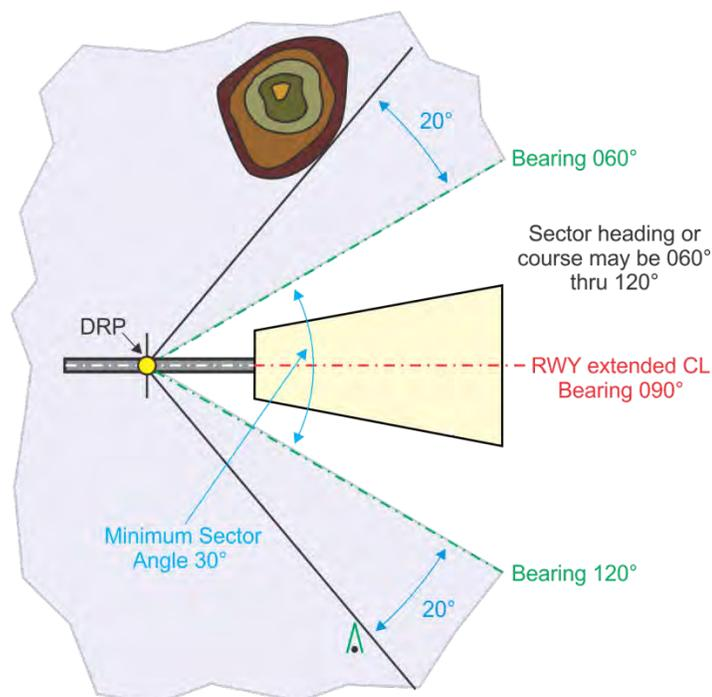
**a.** Boundary based on the ICA. When the 20-degree splay from the DRP cuts across the ICA, construct a line 20 degrees relative to the side of the ICA. To protect the ICA, no obstacle may lie inside this line (see figure 13-2-8).
