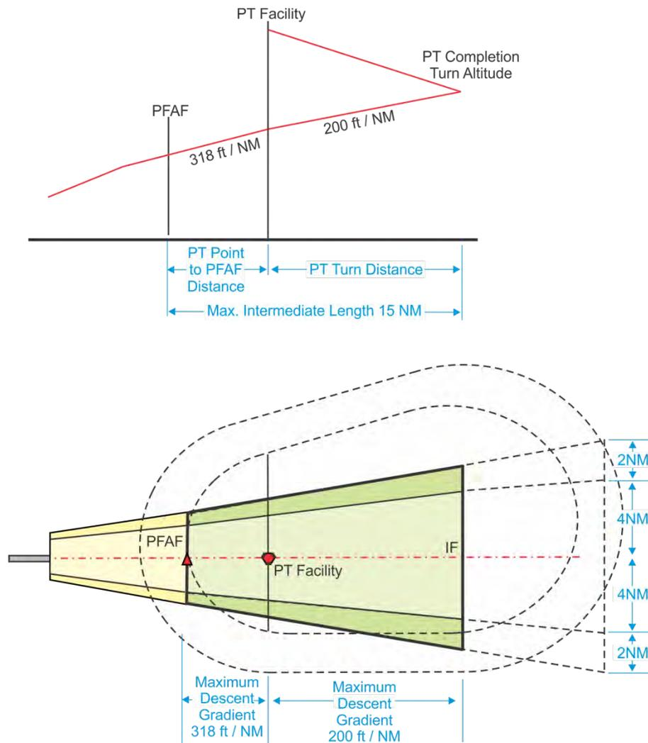
(4) The maximum descent gradient is 200 ft/NM. If the PT facility/fix is a stepdown fix, the descent gradient from the stepdown fix to the PFAF may be increased to a maximum of 318 ft/NM (see figure 2-5-7). The PT distance may be increased in 1-NM increments up to 15 NM to meet descent limitations.
