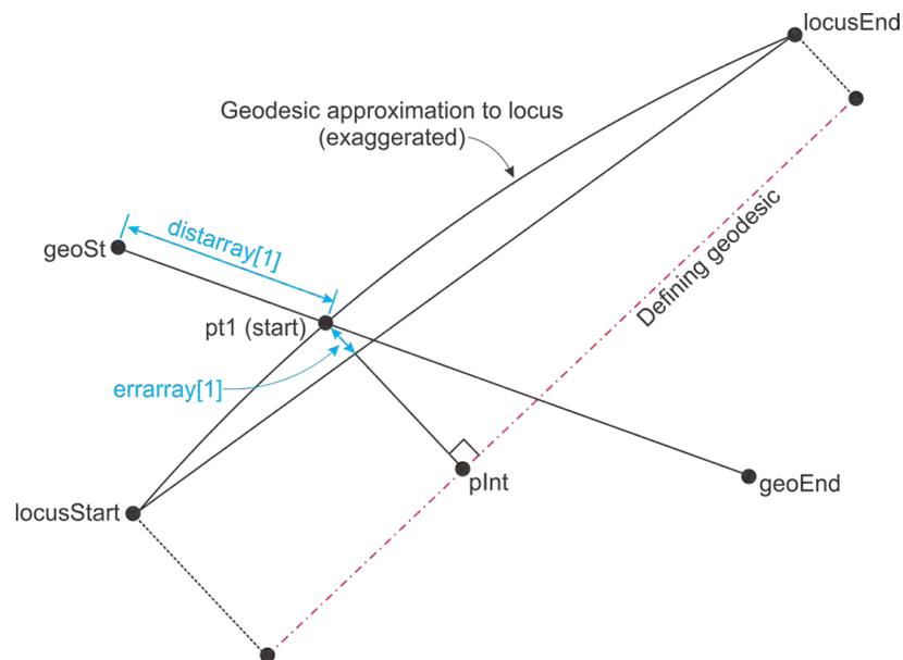
**Figure F-26. Computing First Update to Locus-Geodesic Intersection**
