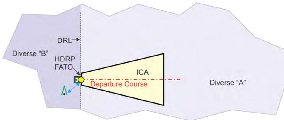
(4) Evaluation of the diverse area for helicopters may be conducted from the helipad in all directions from the FATO utilizing the 20:1 slope from the helipad elevation. If the evaluation reveals all surfaces clear in all directions, then the diverse area is considered clear and standard minimums apply and no departure course will be required. In this case, there is no distinction of Diverse “A” and “B” areas.
