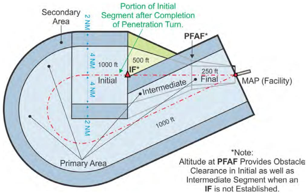
**Figure 5-2-3. Alignment Options for Final Approach Course. Off-Airport VOR with PFAF. Straight-In Approach**
