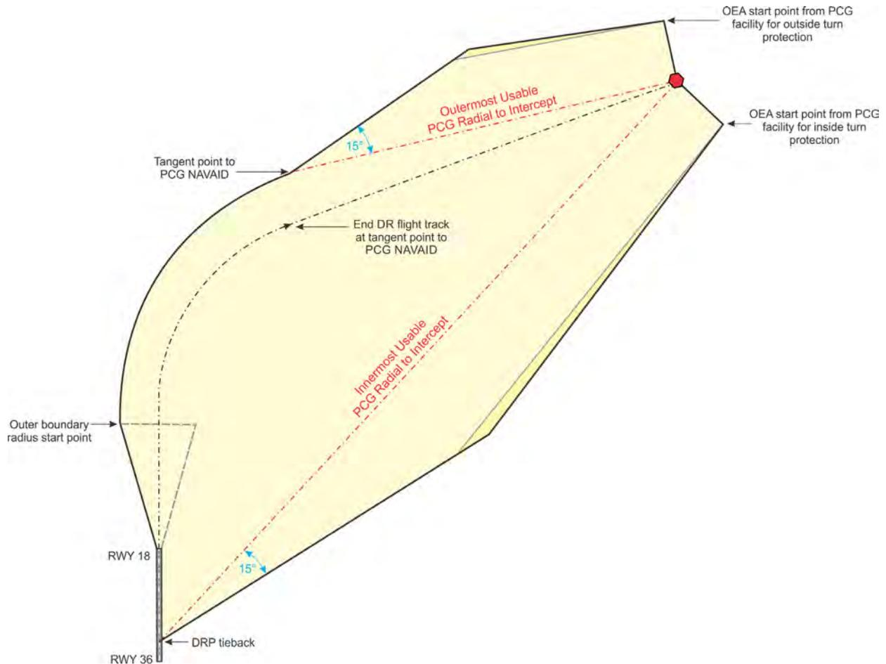
(2) Turn Greater Than 90 Degrees but Less Than or Equal to 180 Degrees, OEA Construction (see figure 13-3-13).
