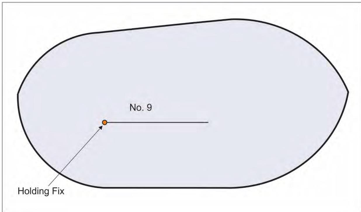
**16-3-3. Altitude Levels.** Table 16-3-1, Holding Pattern Selection Chart, provides holding levels from MHA to FL 500 at intervals of 2000 feet. Holding at 2000 feet and below requires use of the appropriate pattern for 2000 feet. Holding at higher even altitudes requires use of appropriate altitude/flight level patterns as listed in table 16-3-1. Holding at odd altitudes above 2000 feet is determined by use of the next higher even altitude/flight level pattern.
