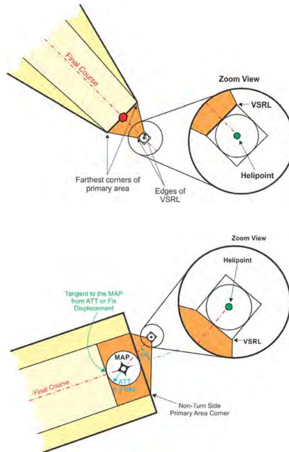
(b) A visual segment descent angle (VSDA) is established from the MAP to the center of the helipad at the desired HCH/hover height. The optimum HCH/hover height is five feet, but may be increased up to 20 feet if necessary to mitigate penetrations of the visual segment surface. The optimum VSDA is six degrees, but may not exceed 7.5 degrees. A VSDA greater than 7.5 degrees may be used with Flight Standards approval.
