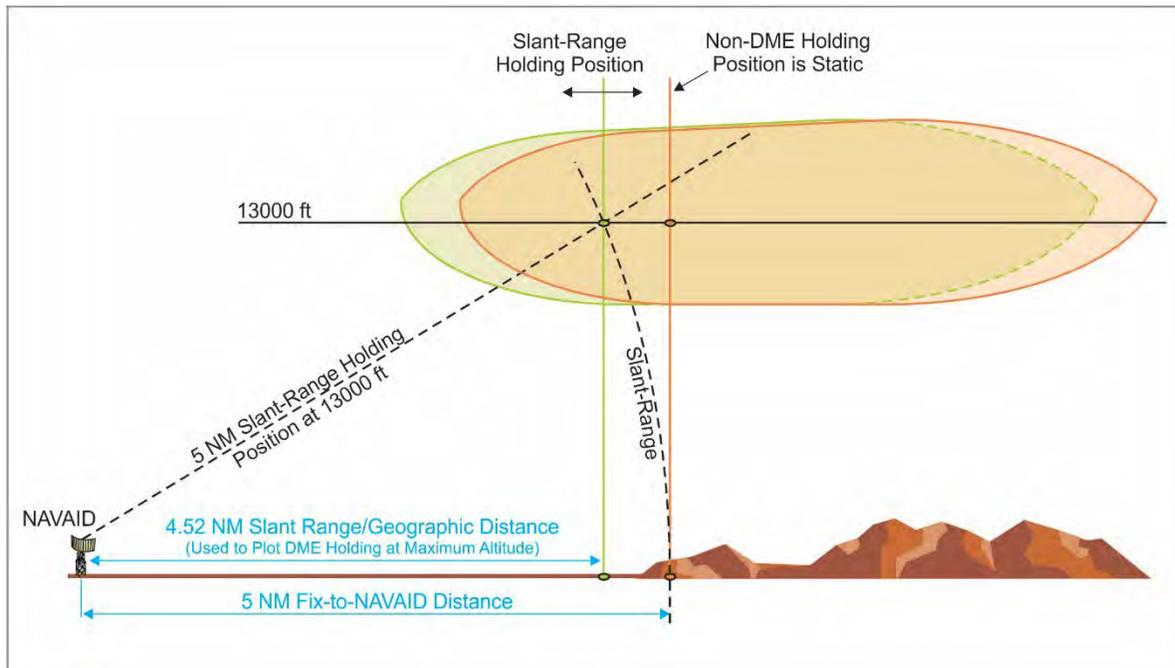
**Note:** Figure 16-4-1 shows holding toward the NAVAID with extended airspace at the fix end when holding away from the NAVAID, the extended airspace would be on the outbound end.
