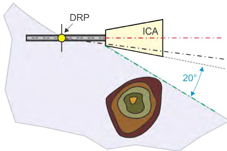
**b.** Outer boundary involving a turn. Locate the turn point on runway centerline (extended) and establish the ICAE. Construct the outer boundary from the ICAE, using table 13-3-2 for selection of the outer boundary radius. Construct a line from the obstacle tangent to the outer boundary radius. Establish the outer boundary buffer 20 degrees from this line on the maneuvering side. Begin the 20-degree buffer at the tangent point where the obstacle line intercepts the arc (see figure 13-2-9).
