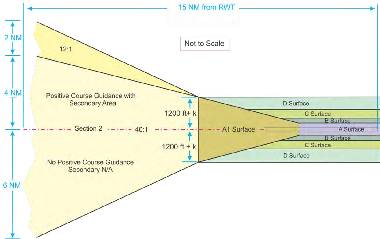
(2) Turning Missed Approach Area (applies to turns of more than 15 degrees) (see figure 10-5-4). Design the procedure to accommodate an aircraft turning at least 400 feet above the TDZE rounded to the nearest foot. Aircraft are assumed to be 200 feet above the runway elevation at the end of the A1 surface; therefore, an extension to the A1 surface must be constructed (referred to as A1<sub>extended</sub>). Determine the length of A1<sub>extended</sub> by applying formula 10-5-4.
