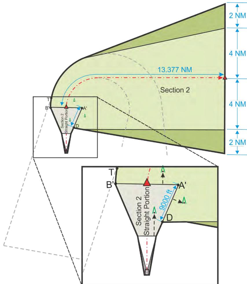
**10-3-4. Missed Approach CG.** Where the section 2 OCS is penetrated and the lowest HAT is required, a missed approach CG greater than standard may be specified. Gradients greater than 425 ft/NM require a waiver. Calculate the required climb gradient termination altitude (CGTA) and the CG by applying formula 10-3-7 and formula 10-3-8.
