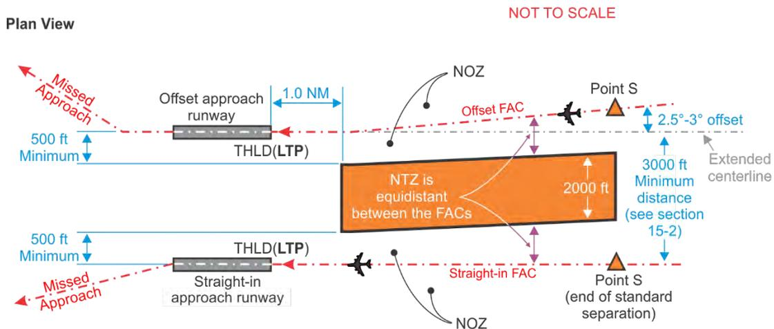
f. Offset FAC. An angular offset of the FAC from the runway extended centerline in a direction away from the NTZ. An offset course increases the NOZ width as distance increases from the runway (see figure E-7).
