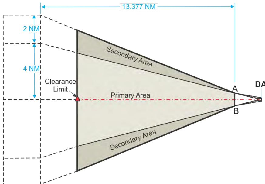
(2) Obstacle clearance. Within the primary area, obstacles are measured shortest distance to line A-B. The section 2 OCS start height is the section 1 OCS end elevation. The standard OCS in the primary area is a 40:1 slope. For obstacles located in the secondary area,
