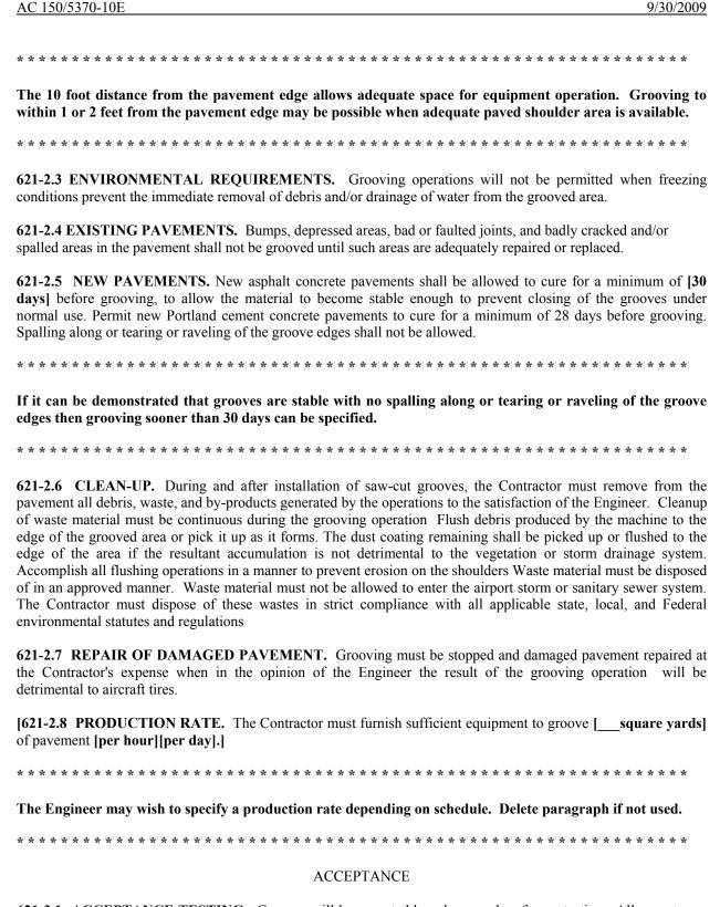
**621-3.1 ACCEPTANCE TESTING.** Grooves will be accepted based on results of zone testing. All acceptance testing necessary to determine conformance with the groove tolerances specified will be performed by the Engineer.
