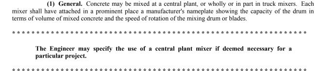
(2) Central plant mixer. Central plant mixers shall conform to the requirements of ASTM C 94.
