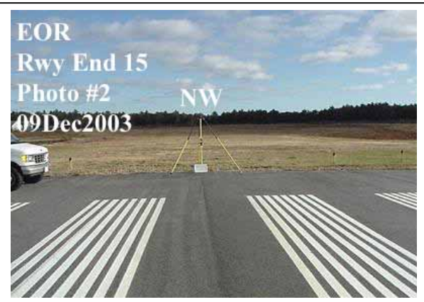
Figure 3-4: Photograph Type #2 (Approach). Photo showing tripod over the mark in foreground and approach in the background.
