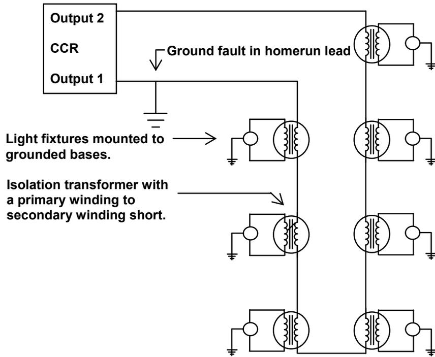
In this failure mode, the light fixture connected to the shorted isolation transformer could produce lethal voltages to anyone touching it.
