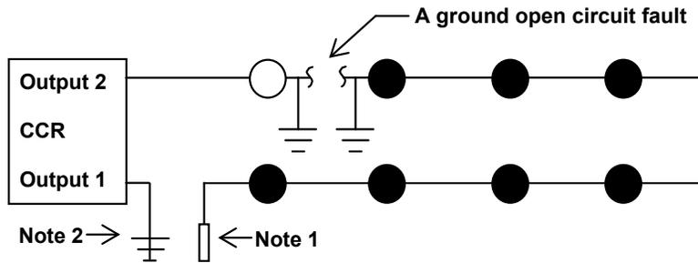
**Figure 6-10a. Grounded Output Test on CCR Output 1**
