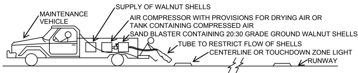
**Figure 5-2. Cleaning Runway Centerline and Touchdown Zone Lights**
