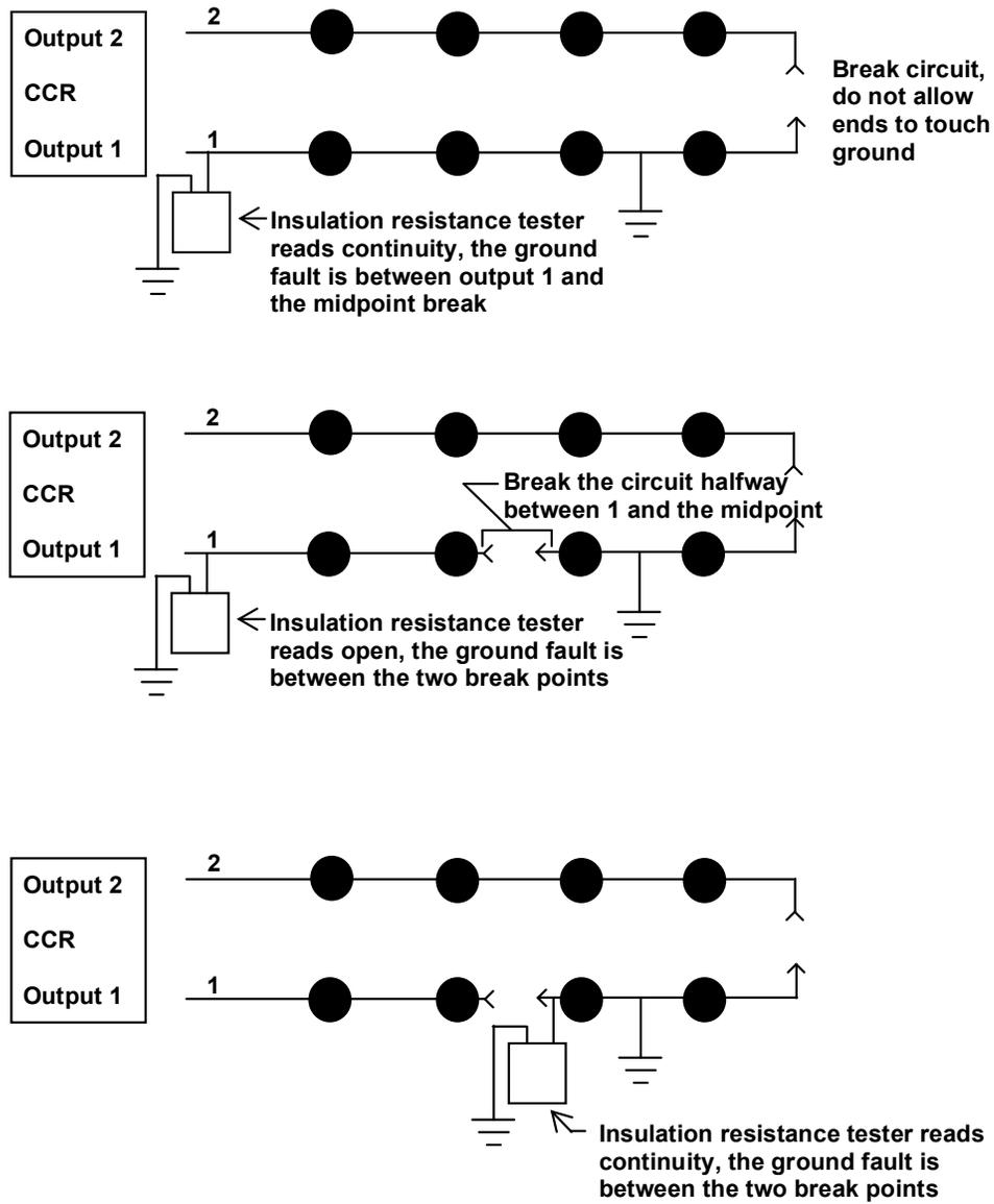
**Figure 6-4. Alternative Method of Finding Ground Fault Using VOM or Insulation Resistance Tester**
