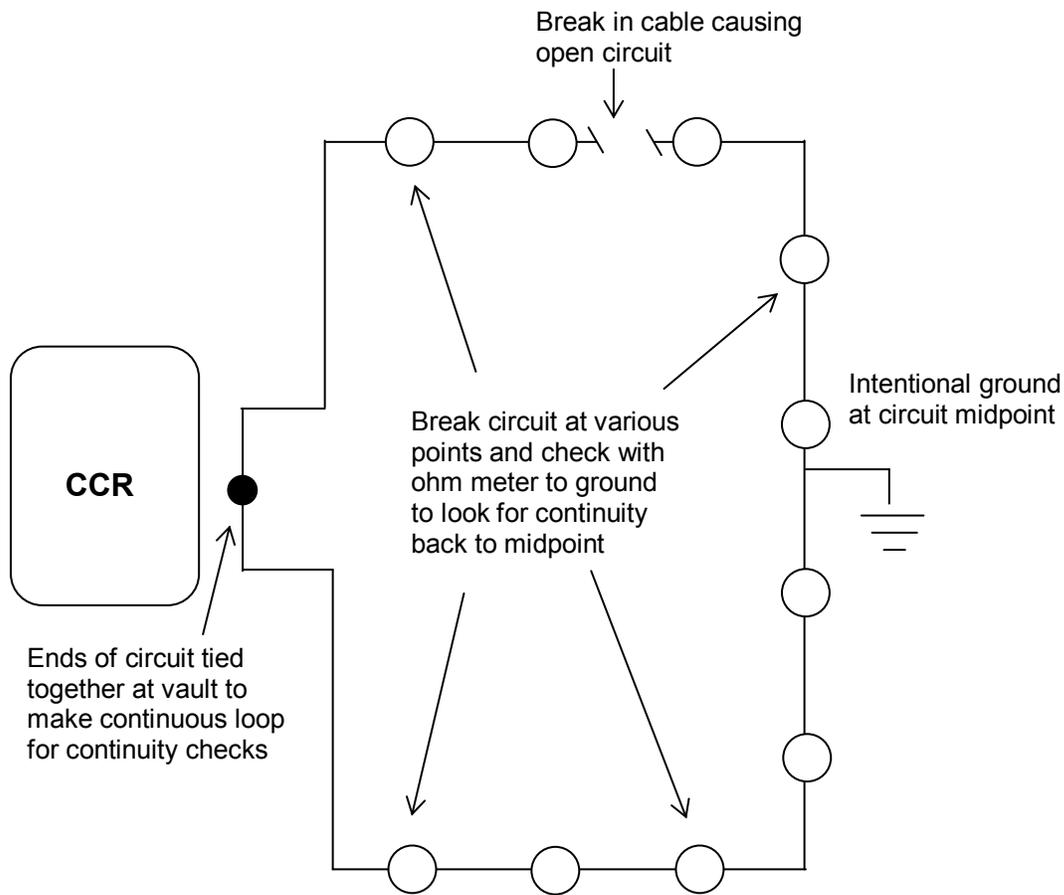
**Figure 6-5. Locating Open Circuit Faults**
