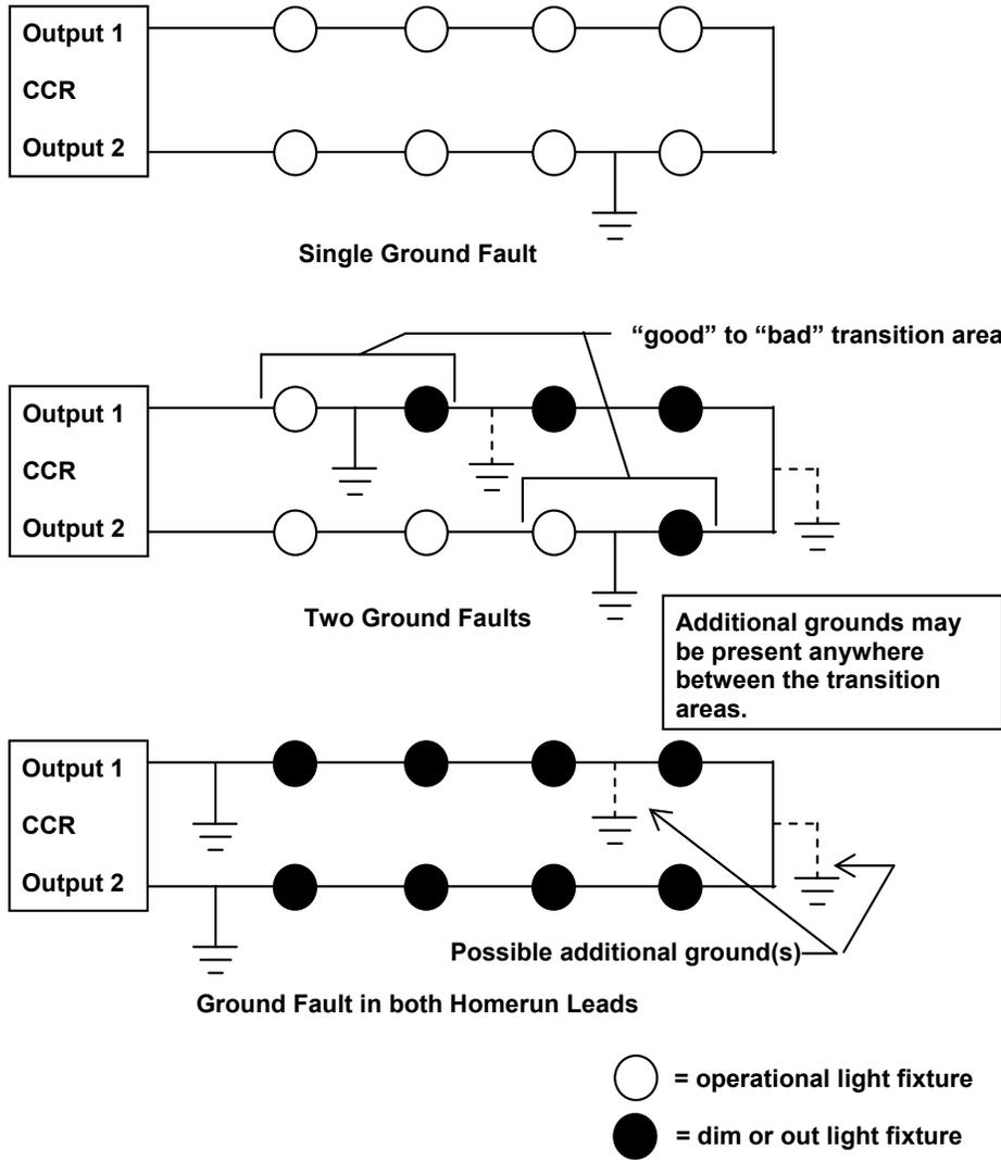
Figure 6-2. Typical Ground Faults
