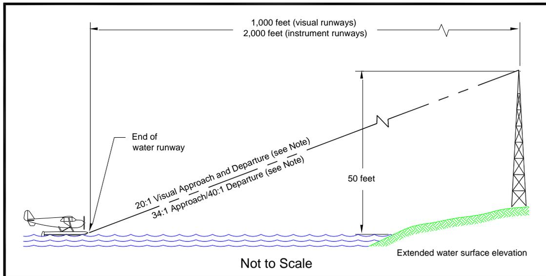
**Note:** The approach and departure surfaces are not individually shown to reduce clutter on graphic. Refer to [AC 150/5300-13](#) to select and site the proper approach and departure surfaces.
