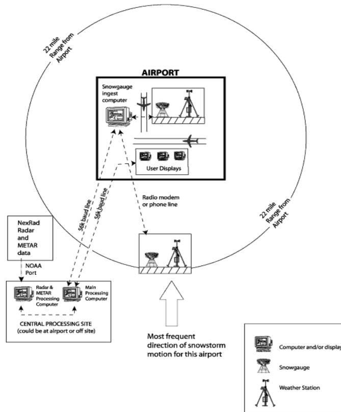
Figure 3-2. Schematic of Unidirectional Storm WSDDM Configuration
