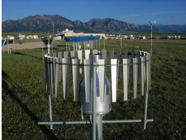
Figure 3-1. Single Alter Wind Shield Type
