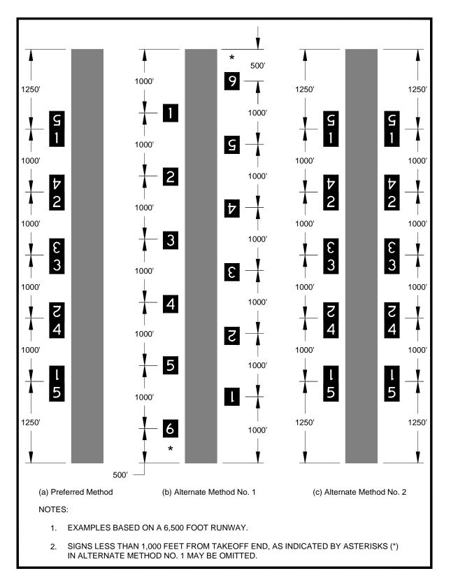
Figure 17. Runway Distance Remaining Sign Configurations.
