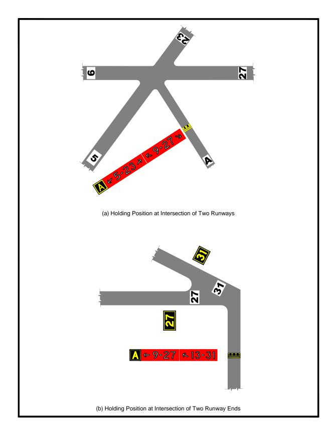
Figure 4. Runway Location Signs and Arrows on Holding Position Signs.
