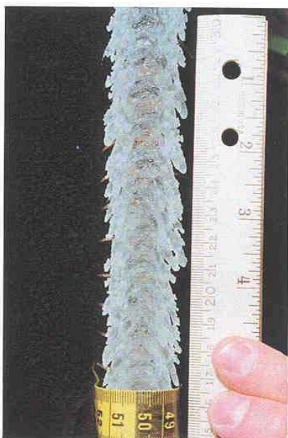
Figure R-20(b). Natural-ice ice accretion (scalloped) obtained with the NASA-GRC Twin Otter ( \Lambda=30^\circ , V=144 mph, T=21^\circ\text{F} , \text{LWC}=0.45 g/m 3 , \text{MVD}=13 \mu\text{m} , t=8 min).
