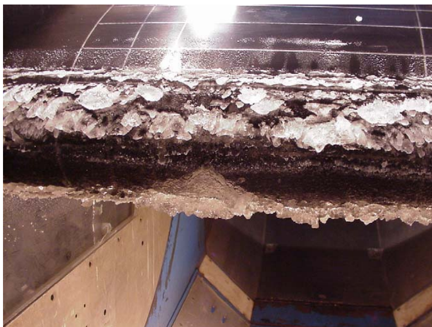
Figure R-4(a) Hybrid NACA 23012 2D (simulating a 72-inch chord airfoil) mode 1 intercycle ice before the third cycle of a pneumatic deicing boot. Three-minute boot cycle intervals were used. The test was performed in 14 CFR part 25, Appendix C Maximum Continuous Icing Conditions. (Static temperature = 14°F, LWC = 0.45 g/m 3 , MVD = 20 micrometers, Spray time = 6:11 min., Tunnel airflow speed = 195 mph, Model AOA = 4°.)
