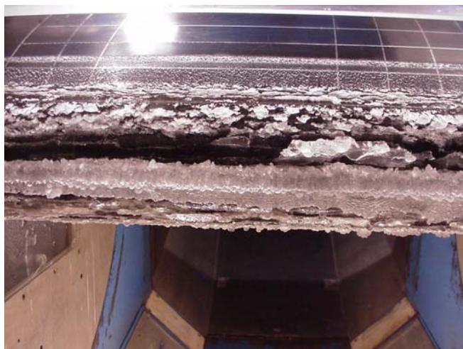
Figure R-4(b). Hybrid NACA 23012 2D (simulating a 72-inch chord airfoil) model intercycle ice before the sixth cycle of pneumatic deicing boot. One-minute boot cycle intervals were used. The test was performed in 14 CFR part 25, Appendix C Maximum Continuous Icing Conditions. (Static temperature = 14°F, LWC = 0.45 g/m 3 , MVD = 20 micrometers, Spray time = 6:11 min., Tunnel airflow speed = 195 mph, Model AOA = 4°.)
