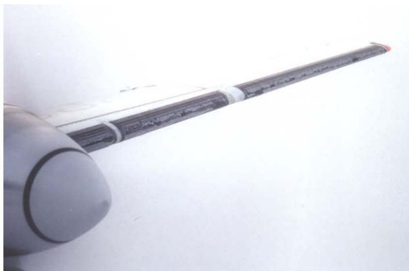
Figure R-6(b). Wing deicing boots intercycle ice accretion photographed during revenue service.
