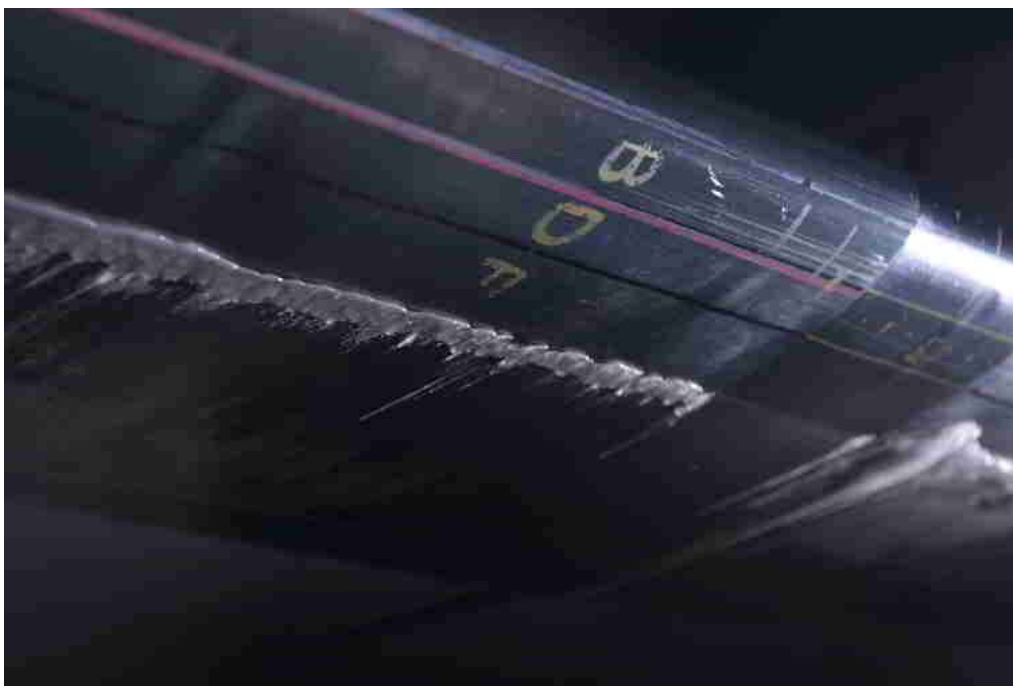
Figure R-9. Lower Surface Runback Ice on a 36-inch NACA 0012 Airfoil Model. The model was equipped with an electro-thermal IPS. The IPS ran wet with a constant protection surface temperature of about 50^{\circ}\text{F} . The mixed-phase icing cloud exposure time was 5 minutes. (Static Temperature = 0^{\circ}\text{F} , LWC = 0.35 \text{ g/m}^3 , MVD = 20 micrometers, IWC (shaved ice) = 0.35 \text{ g/m}^3 , tunnel airflow speed = 120 mph, model AOA = 0^{\circ} ).
